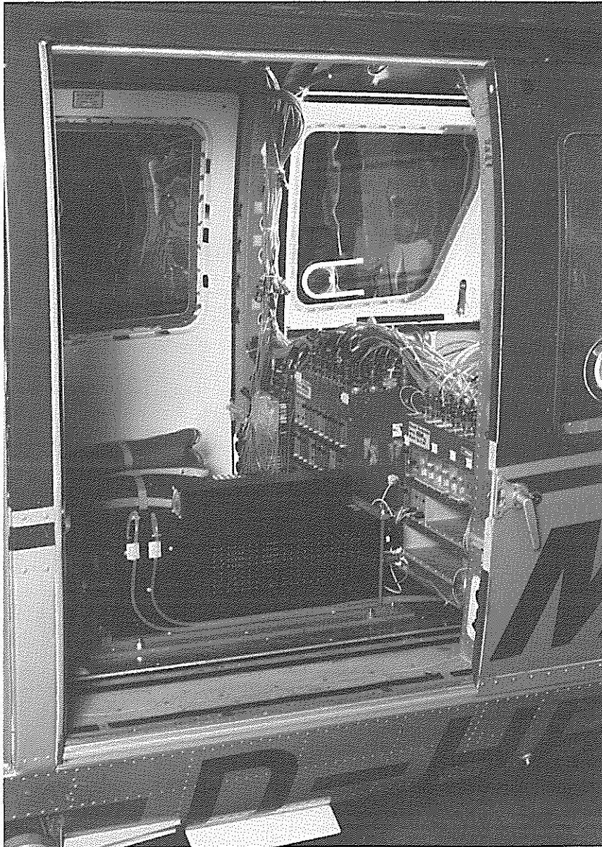
Fig. 7 Installation of the STRAP DOWN Equipment in the Test Helicopter BK117
