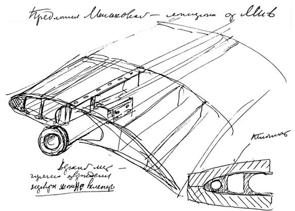
Fig. 5. The sketches of composite blade layout. M.L. Mil was the first to offer a steel tubular spar, combined all the structural members by means of filling them with foamed polyurethane and glassfibre-reinforced plastic.
