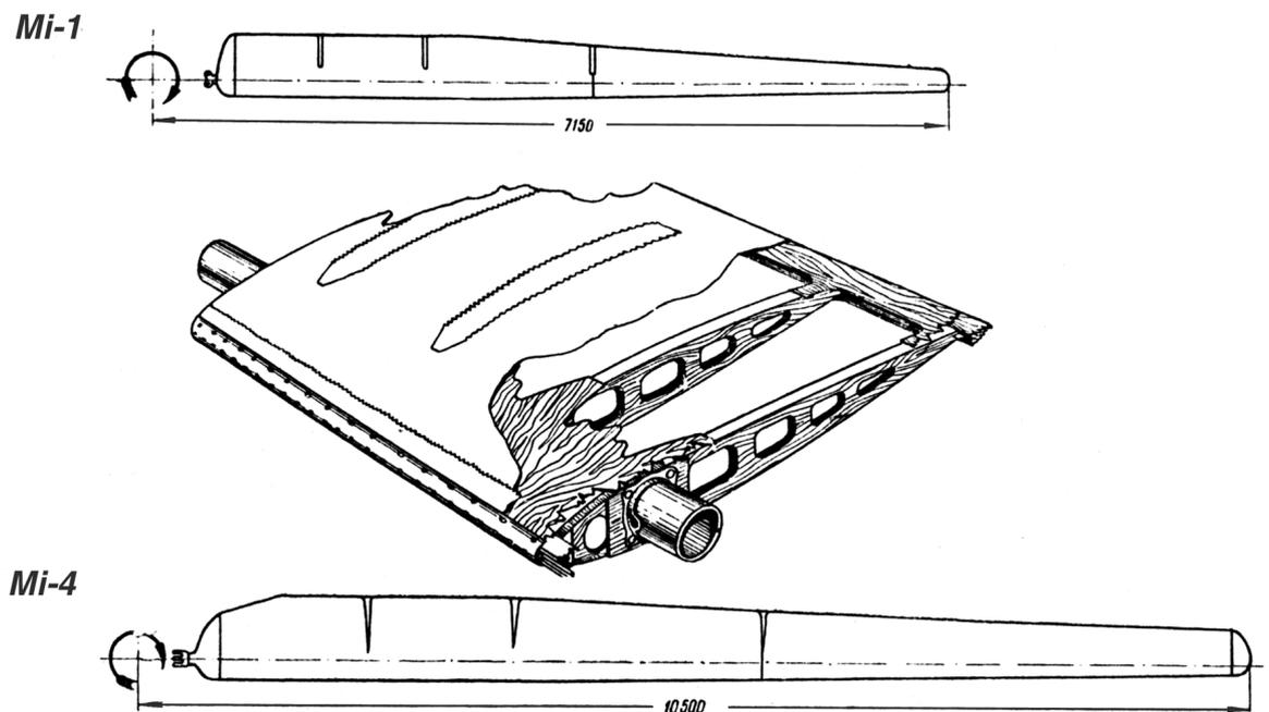
Fig. 2. Blades of mixed construction in the Mi-1 and Mi-4 production helicopters (1949-1956).
