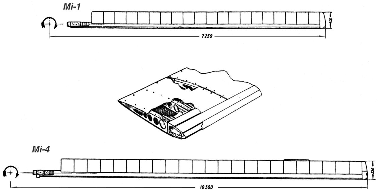
Fig. 3. The blade with a duralumin shaped spar and honeycomb filler of metal foil (1956)
