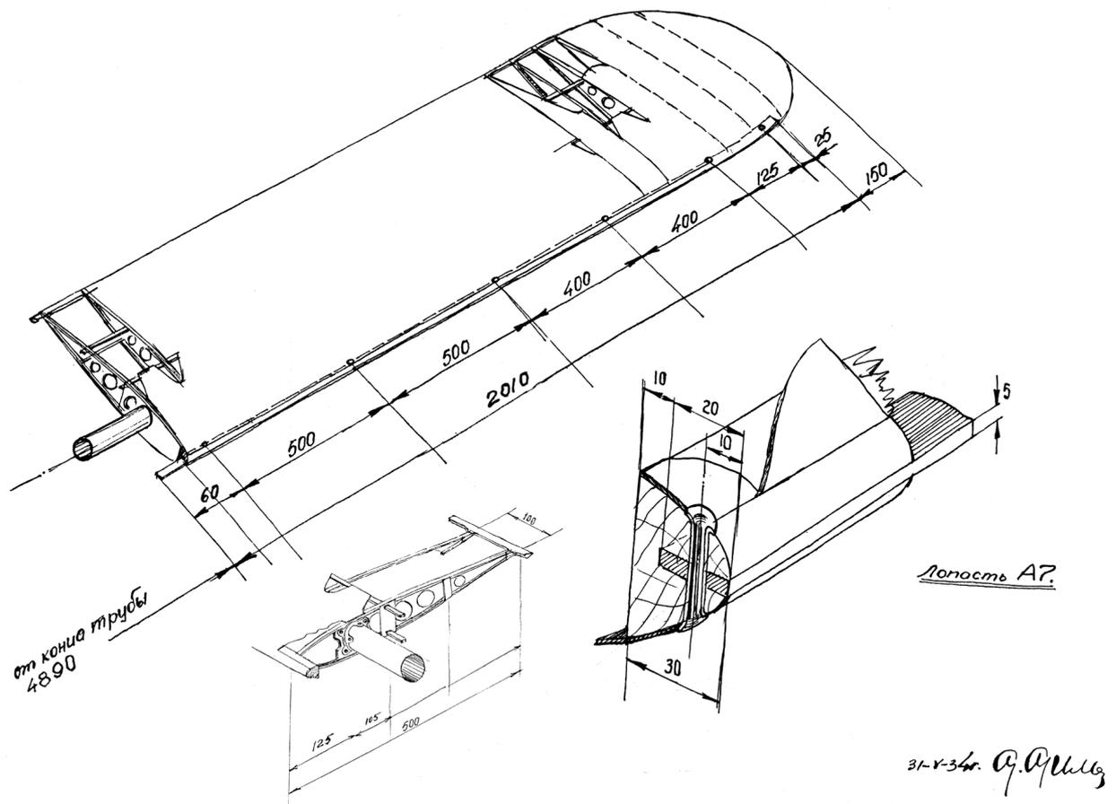
Fig. 1. The A-7 autogiro blade structural analysis: blade, rib, counterweight attachment.
