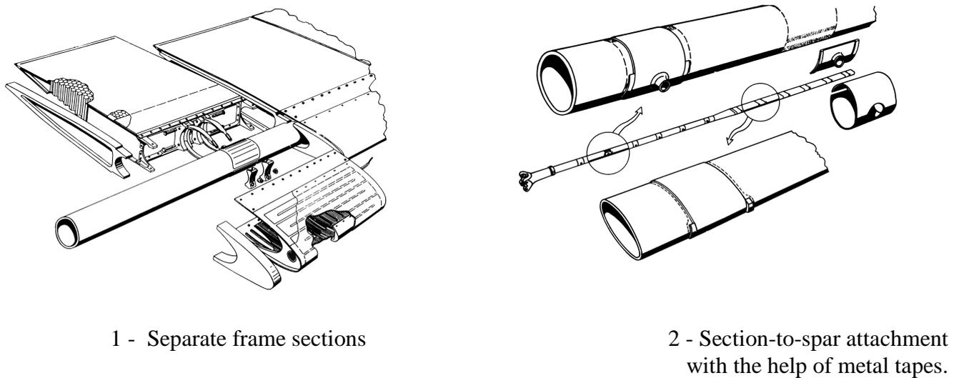
Fig. 4. The Mi-6 blade with single-tube spar
