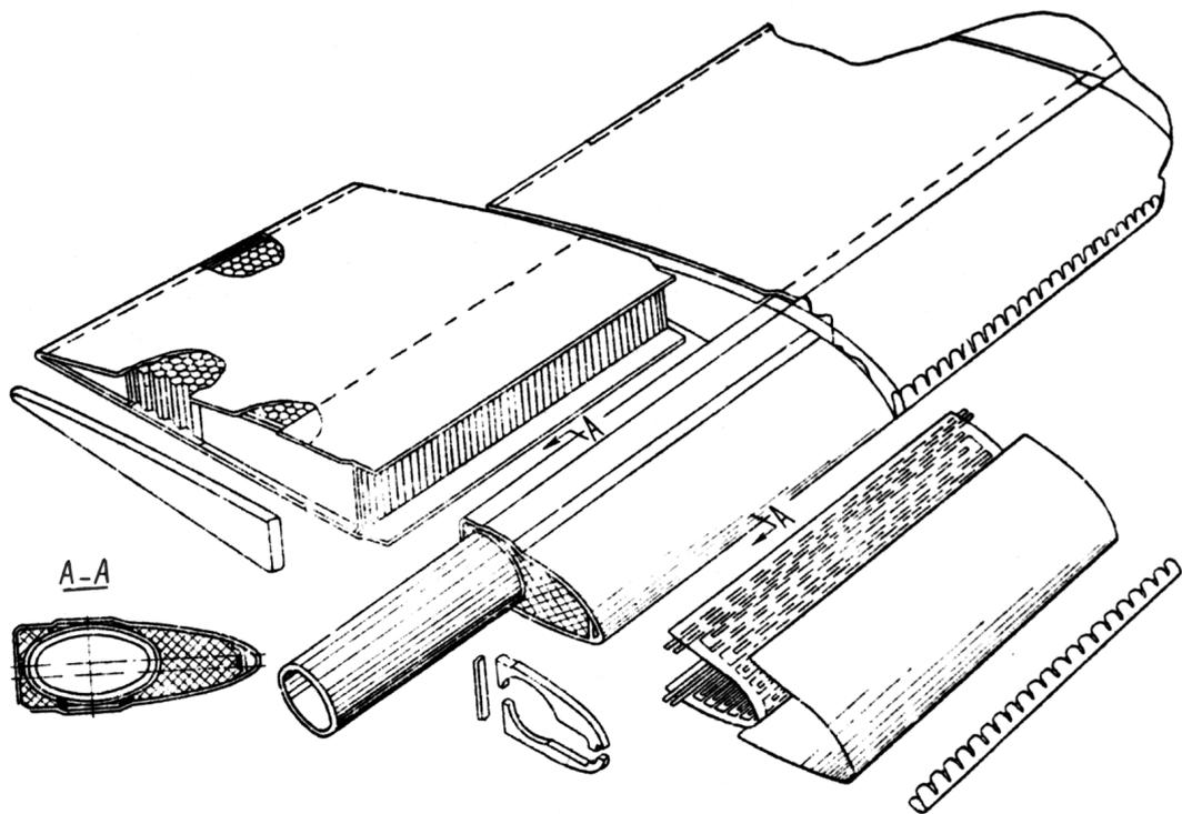
Fig. 6. V-12 Main Rotor Blade. The spar is covered with skin to which nose section frame members are bonded.
