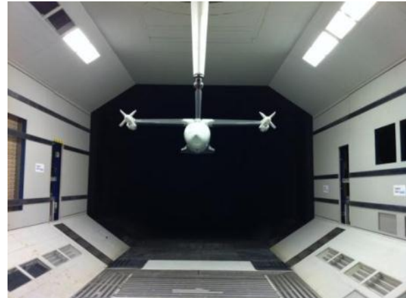
Fig. 3. ERICA model in RUAG LWTE Test Section – Front View
