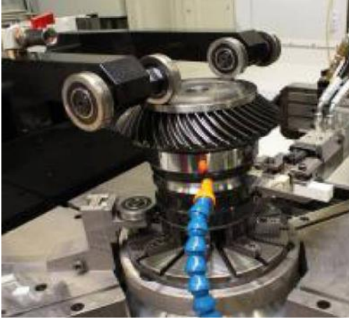
Figure 28: Honing Process on a Gear Raceway
