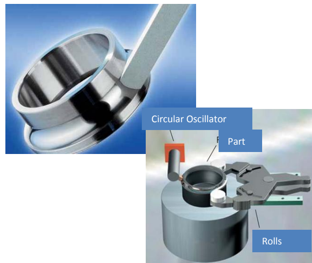
Figure 27: Race Way Honing Process
