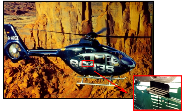
Fig. 18: Helicopter EC135 with detail showing opened service step
