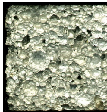
Fig. 17: Fracture Surface Specimen: HAL 175/4/1 22s Number of cycles: 1,195,475 Stress/density: 3,34 MPa/(g/cm 3 ) Density: 0.299 g/cm 3
