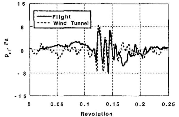
Figure 8. Flight and wind tunnel comparison of averaged time histories for 1/4 revolution (Ref. 9). Flight pt. 307 conditions:  $C_T = 0.00605$ ,  $M_{tip} = 0.606$ ,  $\mu = 0.203$ ,  $\alpha_{app} = 0.5$  deg. Wind Tunnel Run 48\_19 conditions:  $C_T = 0.00599$ ,  $M_{tip} = 0.605$ ,  $\mu = 0.200$ ,  $\alpha_{app} = 0.0$  deg.
