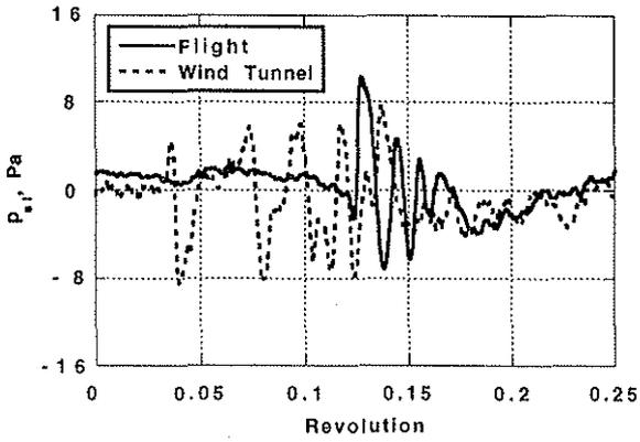
Figure 9. Flight and wind tunnel comparison of averaged time histories for 1/4 revolution (Ref. 9). Flight pt. 315 conditions:  $C_T = 0.00600$ ,  $M_{tip} = 0.606$ ,  $\mu = 0.254$ ,  $\alpha_{tip} = 0.4$  deg. Wind Tunnel Run 48\_18 conditions:  $C_T = 0.00597$ ,  $M_{tip} = 0.605$ ,  $\mu = 0.251$ ,  $\alpha_{tip} = 0.0$  deg.
