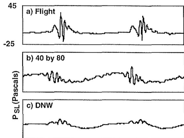
Figure 13. Acoustic pressure time histories for 1/2 revolution (Ref. 10). Condition #1;  $\alpha_{tip} \approx 2.4$  deg,  $\mu \approx 0.185$ ,  $C_w \approx 0.00465$ ,  $M_{tip} \approx 0.64$ , a) Flight, b) 40-by 80, c) DNW.
