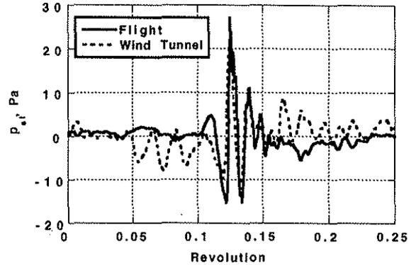
Figure 7. Flight and wind tunnel comparison of averaged time histories for 1/4 revolution (Ref. 9). Flight pt. 203 conditions:  $C_T = 0.00778$ ,  $M_{tip} = 0.603$ ,  $\mu = 0.164$ ,  $\alpha_{app} = 5.6$  deg. Wind Tunnel Run 39\_24 conditions:  $C_T = 0.00753$ ,  $M_{tip} = 0.605$ ,  $\mu = 0.173$ ,  $\alpha_{app} = 5.0$  deg.
