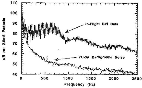
Figure 4. Frequency spectrum of YO-3A background noise and typical BVI data (Ref. 10).
