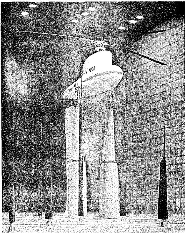
Figure 6. The S-76 rotor installed on the RTA in the 80-by-120-Foot Wind Tunnel.
