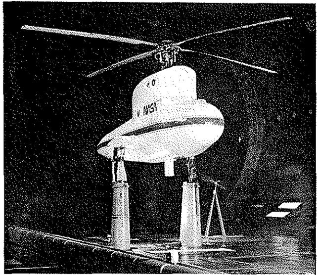
Figure 12. The BO 105 rotor installed on the RTA in the 40-by 80-Foot Wind Tunnel.
