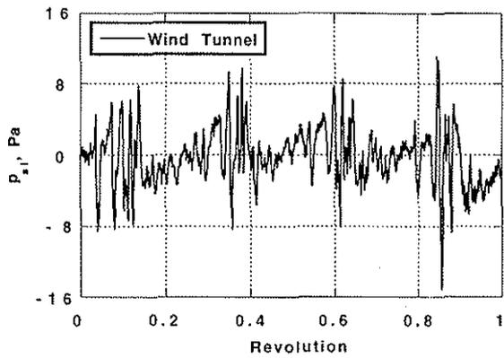
Figure 10. Wind tunnel blade-to-blade variability seen at the higher advance ratio (Ref. 9). Run 48\_18 conditions:  $C_T = 0.00597$ ,  $M_{tip} = 0.605$ ,  $\mu = 0.251$ ,  $\alpha_{tip} = 0.0$  deg.
