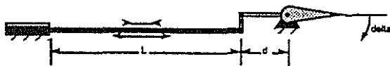
Figure 8: Schematic configuration of bimorph and flap geometry, L =length of bimorph bender beam, d =flap lever arm length [20]
