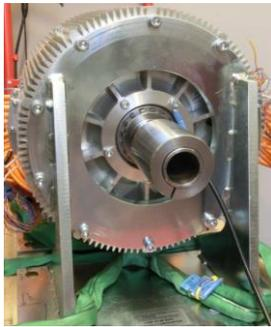
a) Axial-flux prototype including dynamometer mounting arrangement
