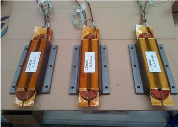
Figure 7. Example motorettes used to calibrated the thermal analyses
