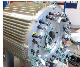
b) End view indicating the independent coil connections
