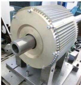
a) Radial-flux prototype including dynamometer mounting arrangement
