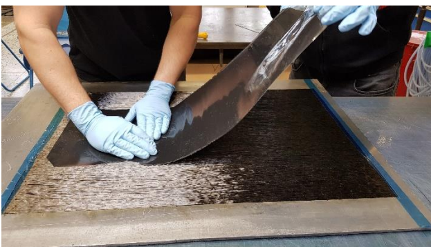
Figure 7: Manufacturing EPDM test specimen with CFRP fiber blanket
