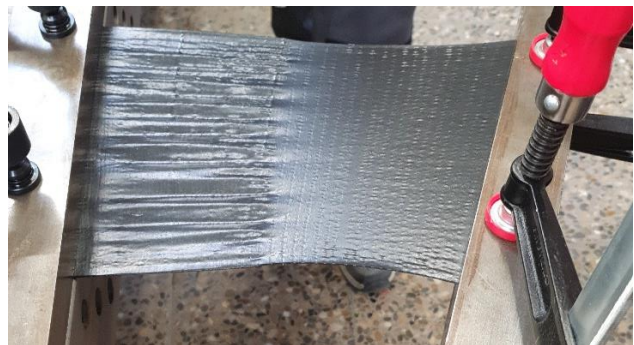
Figure 9: Tensile test of single CFRP fibers strands with different distances in the EPDM skin (left: 1mm, right: 5mm)
