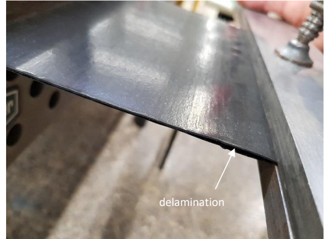
Figure 11: CFRP fibers blanket in the EPDM skin before tensile test
