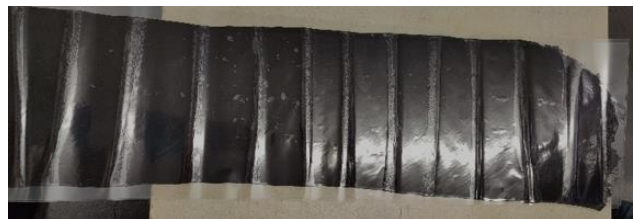
Figure 5: EPDM skin with kinks in the carrier film
