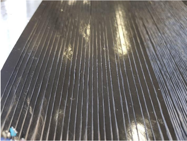
Figure 6: Implementing single CFRP fibers strands with different distances in the EPDM skin
