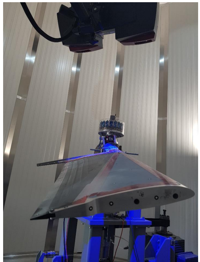
Figure 19: optical outer surface investigation of demonstrator with 30% chord extension
