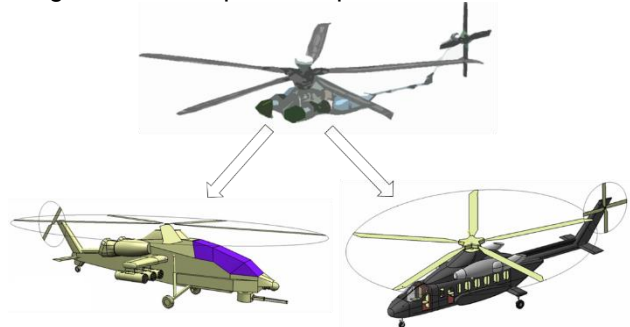
Figure 6: Representation of High-level Commonality for an Attack and a Transport Helicopter
