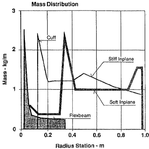
Fig. 3.4 Mass Distribution of the 4-Bladed BK 117 Tail Rotors
