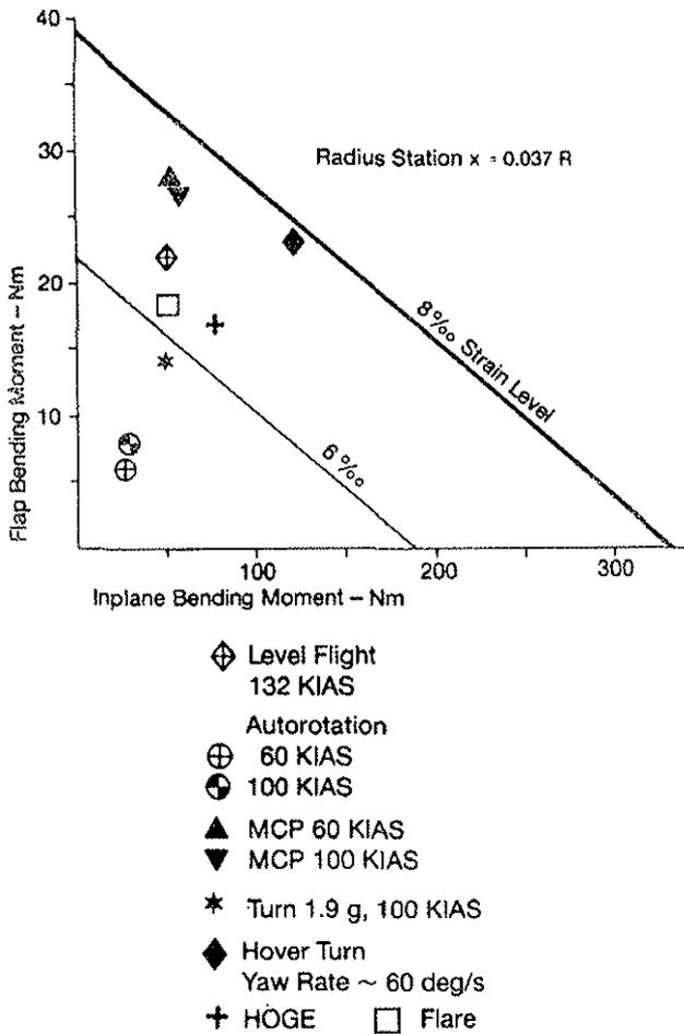
Fig. 4.6 Strain Level in the Flapping Flexure of the 4-Bladed Soft Inplane BK 117 BTR
