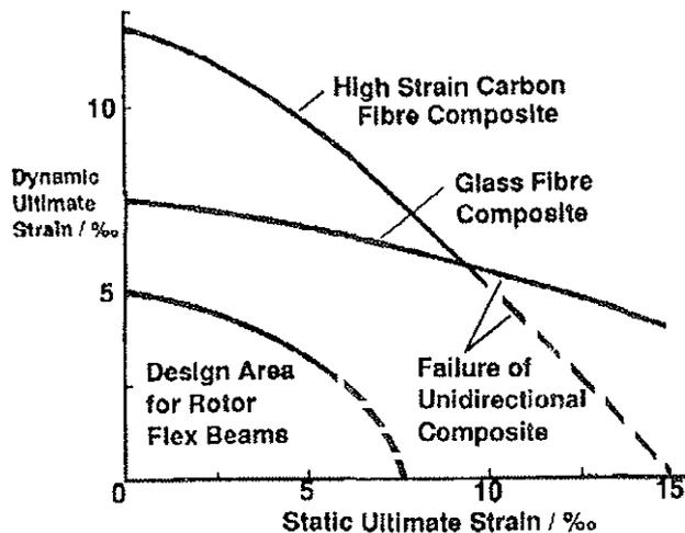
Fig. 5.3 Margin Between Design Area and Failure Limits of Rotor Flexbeams
