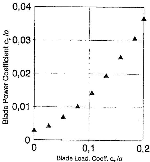
Fig. 4.2 Thrust/Power Characteristics of the Four-Bladed 1,95 m Diameter BK 117 (Growth) BTR (experimental version)
