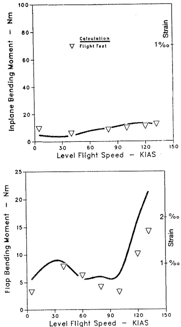
Fig. 4.5 Dynamic Flap and Lead Lag Bending Moment at the Blade Root of the 4-Bladed Soft Inplane BK 117 BTR
