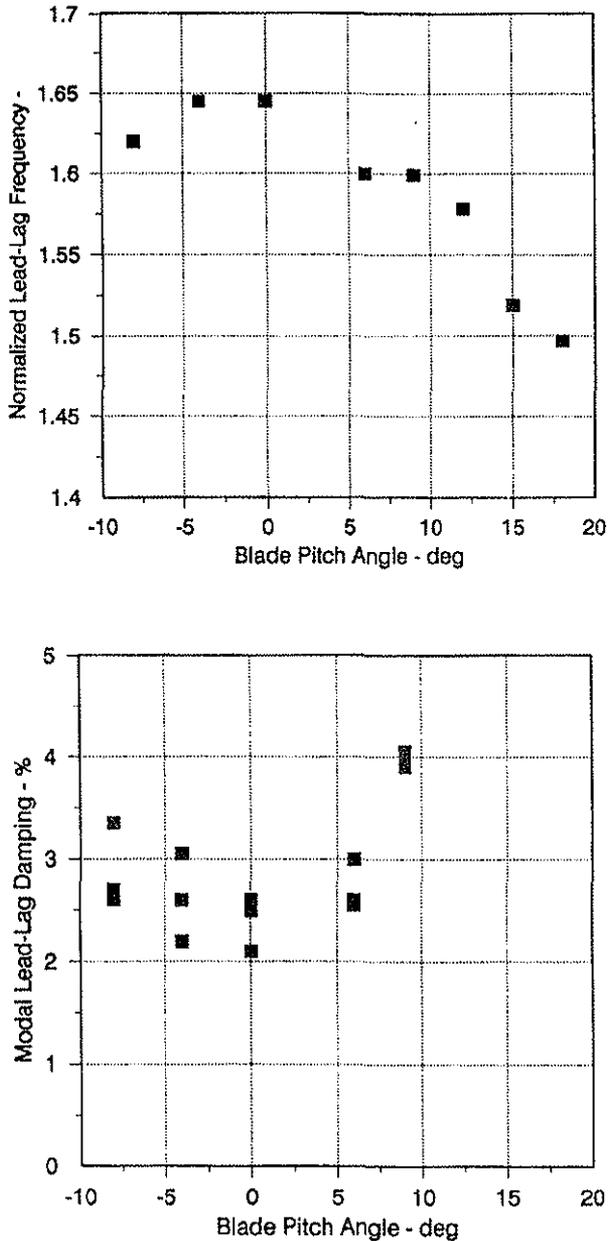
Fig. 4.4 Lead-Lag Mode Frequency and Damping of the 4-Bladed Stiff Inplane BK 117 (Growth) BTR at Nominal Rotor Speed
