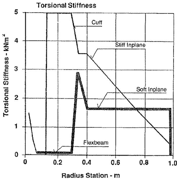
Fig. 3.5 Torsional Stiffness Distribution of the 4-Bladed BK 117 Tail Rotors
