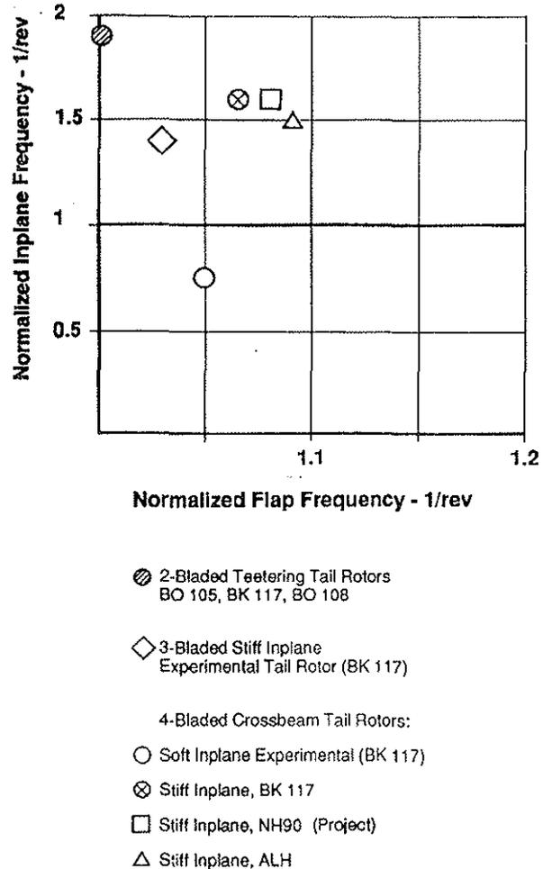
Fig. 3.1 Fundamental Flap and Lead-Lag Frequencies of MBB Tail Rotors
