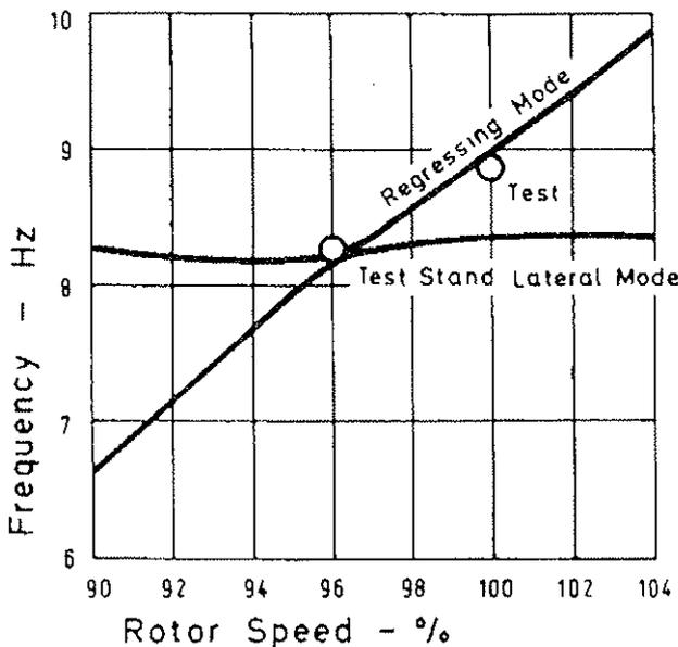
Fig. 3.7 Ground Resonance Simulation of the Soft Inplane Rotor on Whirl Tower
