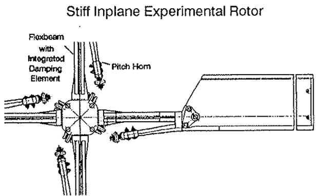
Fig. 3.3 Comparison of Control Devices and Soft and Stiff Inplane Principle
