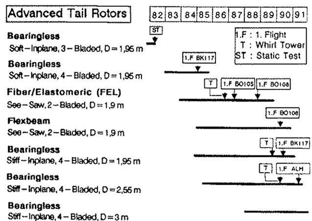
Fig. 1.1 Development and Test of Advanced Composite Tail Rotors at MBB
