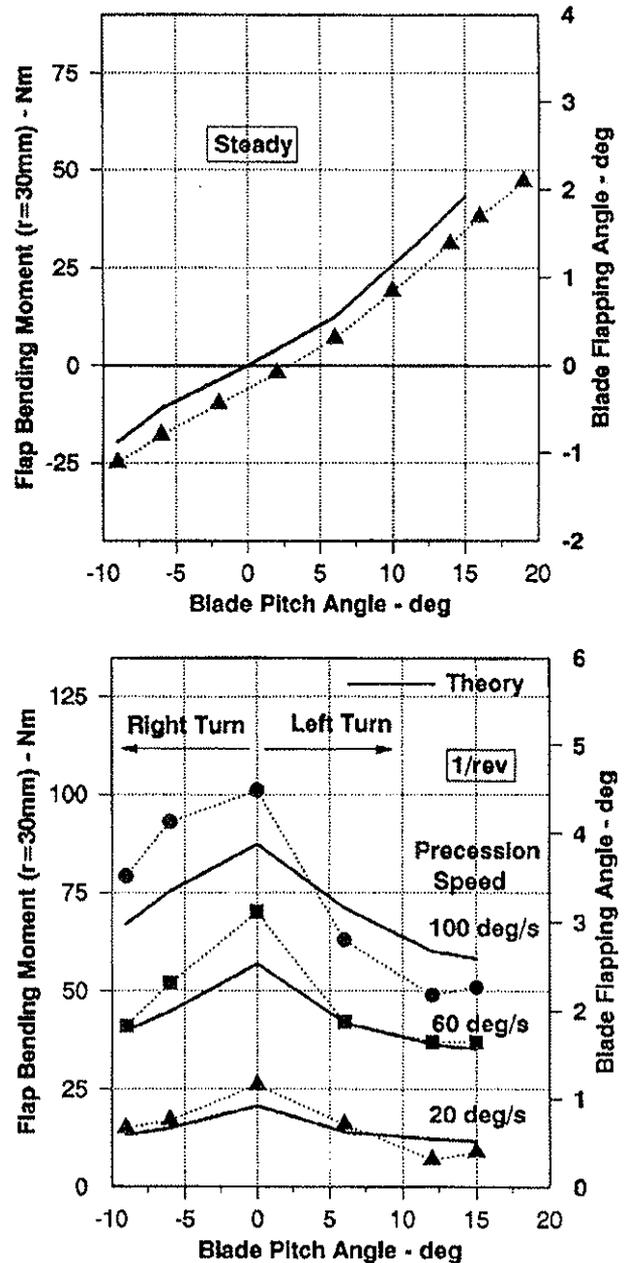
Fig. 4.3 Flap Bending Moment during Precession Tests on the Whirl Tower of the 4-Bladed Stiff Inplane BK 117 BTR
