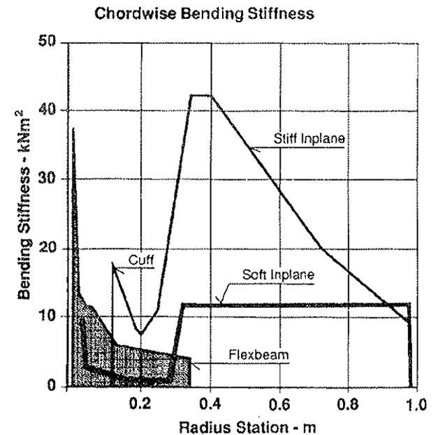
Fig. 3.6 Bending Stiffness Distribution of the 4-Bladed BK 117 Tail Rotors
