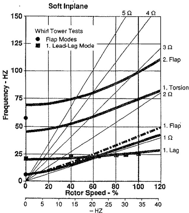
Fig. 3.2 Resonance Diagrams of 4-Bladed BK 117 Experimental BTR's
