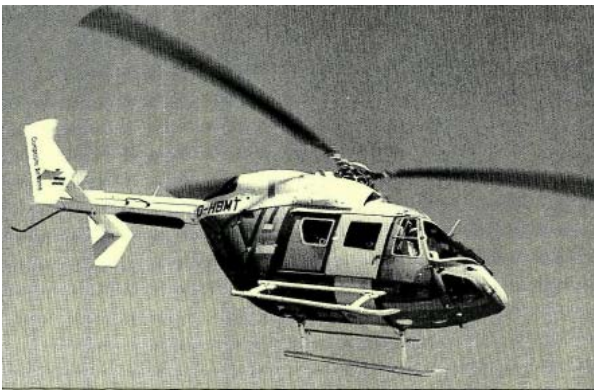
Fig.1: BK117 composite airframe demonstrator
