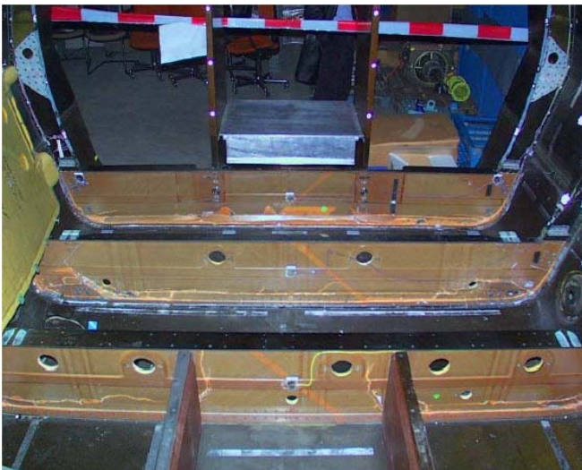
Fig.15: Energy absorption zones at SFG, picture taken after test.
