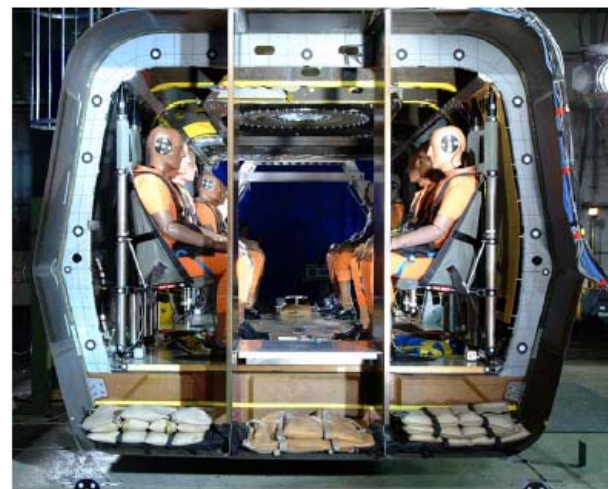
Fig.14: Centre fuselage crash test article, fully equipped, front view.
