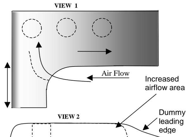
Figure 7. Final/optimal standard of ACS inlet cowl
