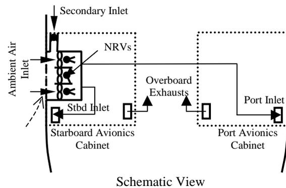
Figure 2. Isometric View and Schematic View of the EH101 Avionics Cooling System
