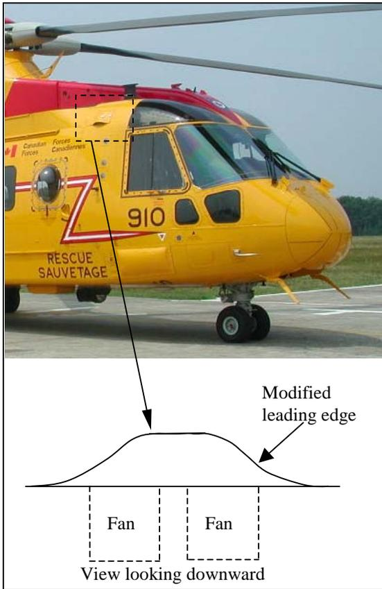
Figure 4. EH101 CSH with the re-shaped ACS inlet cowl
