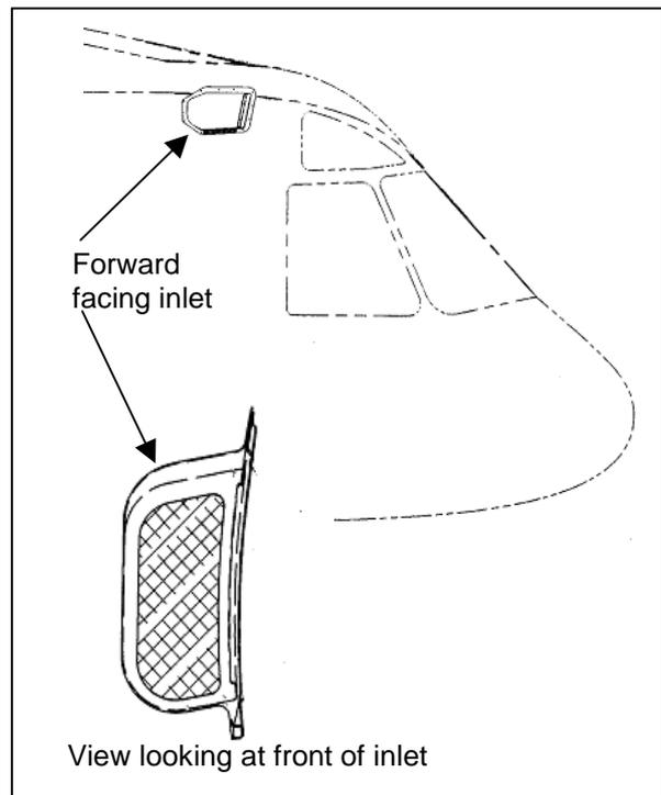
Figure 8. Forward facing ACS Inlet on the EH101 Civil
