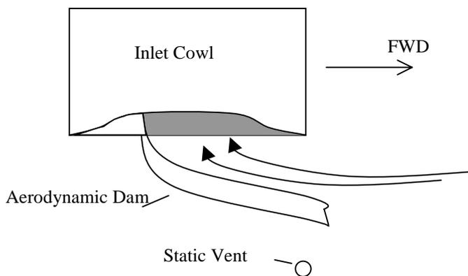
Figure 5. Aerodynamic dam fitted to the original ACS inlet cowl
