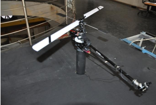
Fig. 4. The investigated helicopter T-REX 450 over the simulated heliport
