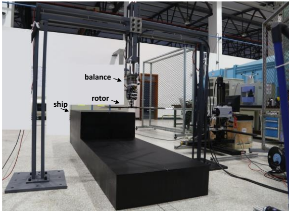
Fig.1 Configuration of rotor and ship interference experiment
