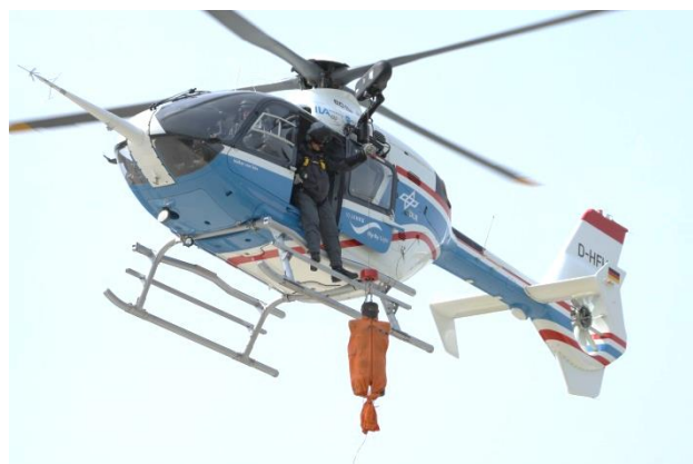
Figure 1: ACT/FHS in flight test with externally slung load and rescue hoist
