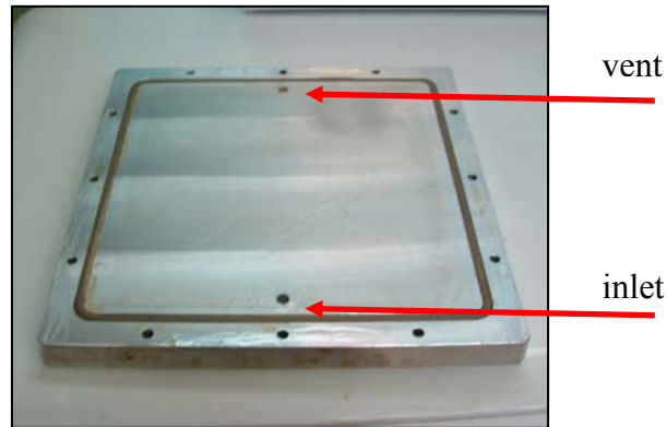
Fig12: half-mold used for process ability test.
