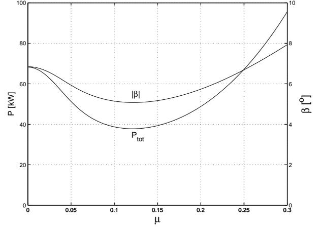
Figure 10: Flap forcing power required and flapping angle for typical light helicopter.
