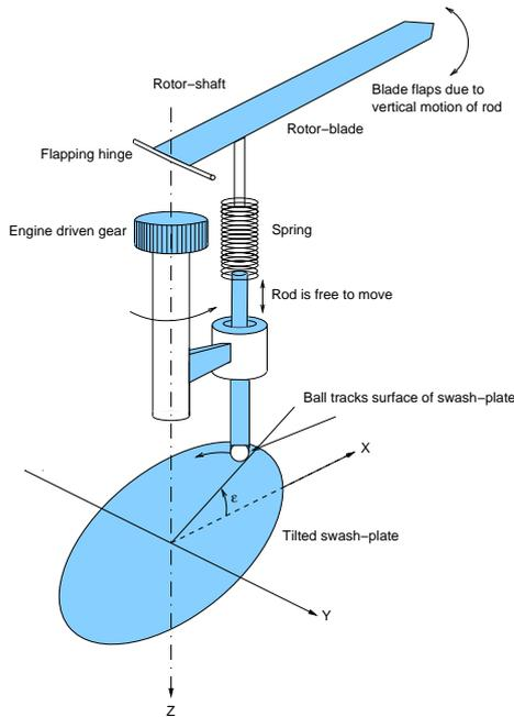
Figure 12: Alternative flap forcing mechanism.
