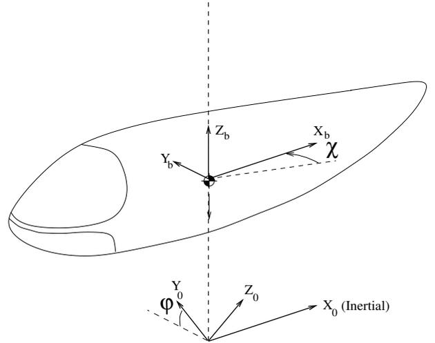
Figure 15: Dynamic model for roll and pitch.
