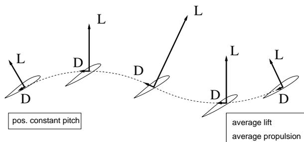
Figure 3: Flapping wing with a constant pitch angle.
