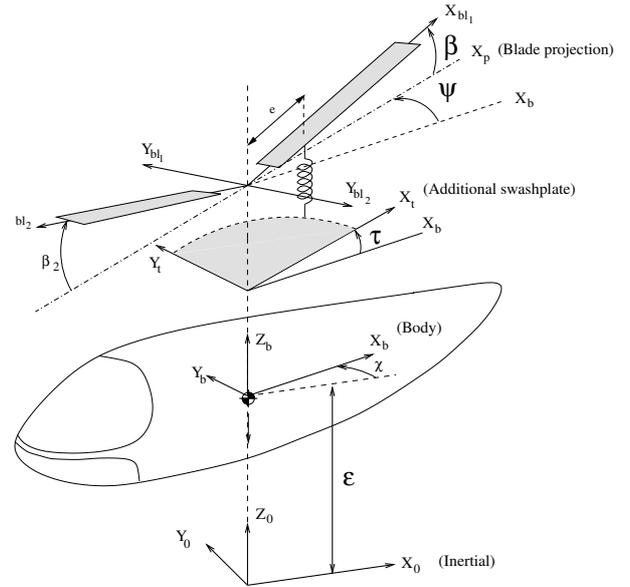
Figure 11: Dynamic model for analyzing vertical vibrations.
