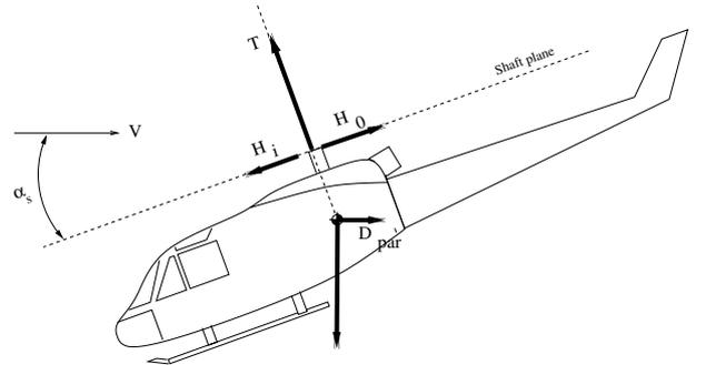
Figure 7: Equilibrium of forces in steady horizontal flight.
