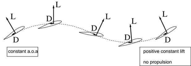
Figure 4: Flapping wing with a constant angle of attack.
