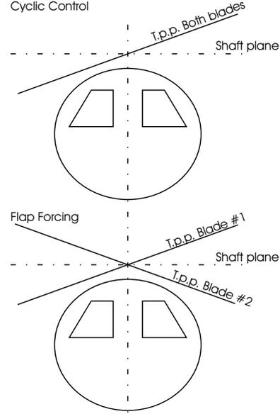
Figure 9: Split of tip path plane due to flap forcing.
