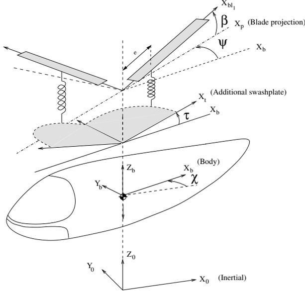
Figure 14: Dynamic model for analyzing yaw vibrations, double teeter.
