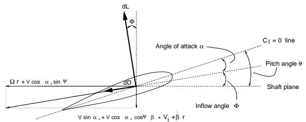
Figure 5: Velocity diagram of blade element.
