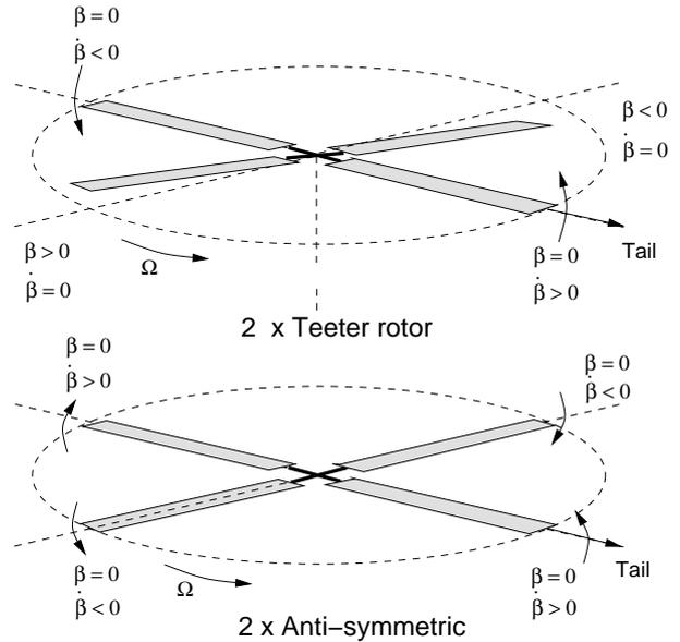
Figure 13: Four-bladed configurations to eliminate vertical vibrations: a) Double teeter, b) Twice two-bladed configuration according to fig.6, in opposite phase.
