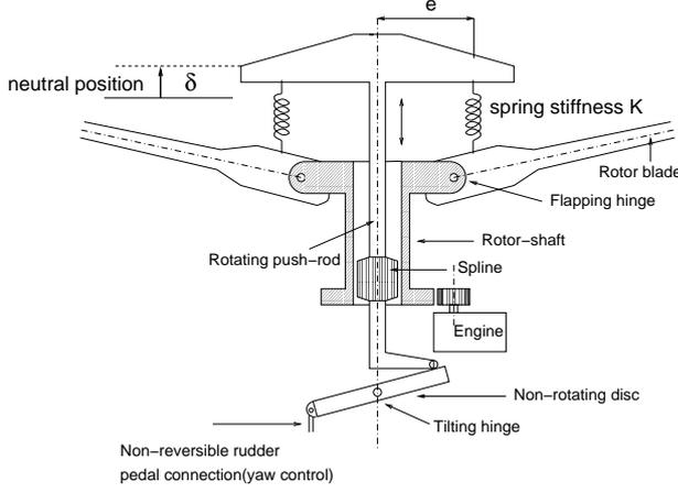
Figure 6: Principle of a possible mechanism for flap forcing.
