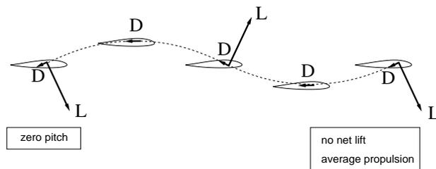
Figure 2: Flapping wing with a pitch angle equal to zero.
