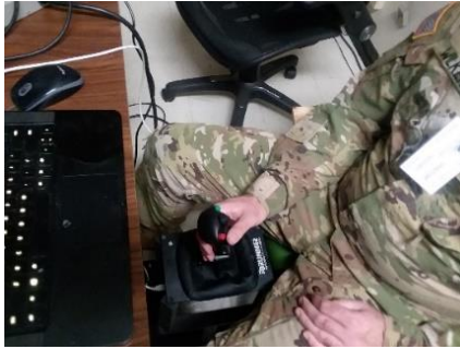
Figure 4. Brunner active inceptor positioned for center-stick use.
