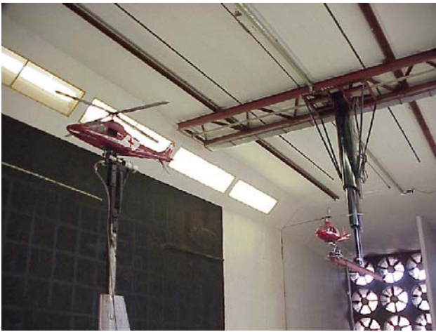
Figure 1 The two RC helicopter models in the wind tunnel with the upwind helicopter on a fixed strut and the downwind helicopter on the traverse system
