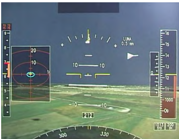
Figure 13: Presentation of the UAV (here: LUNA) on the helicopter's 3D synthetic vision system (SVS)
