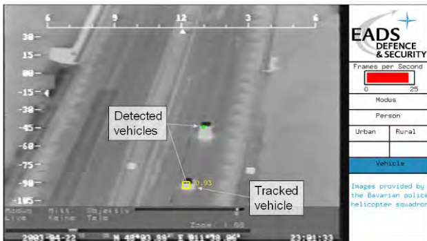
Figure 10: Sensor Graphical user interface of the mobile exploitation station showing a sample image provided by the Bavarian police helicopter squadron.
