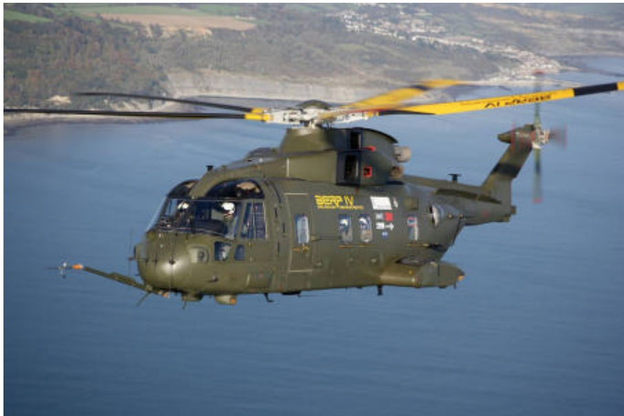
BERP IV Technology Demonstrator Blades on ZJ117, the Merlin HC Mk3 Demonstrator aircraft, over the Dorset Coast in Oct 07
