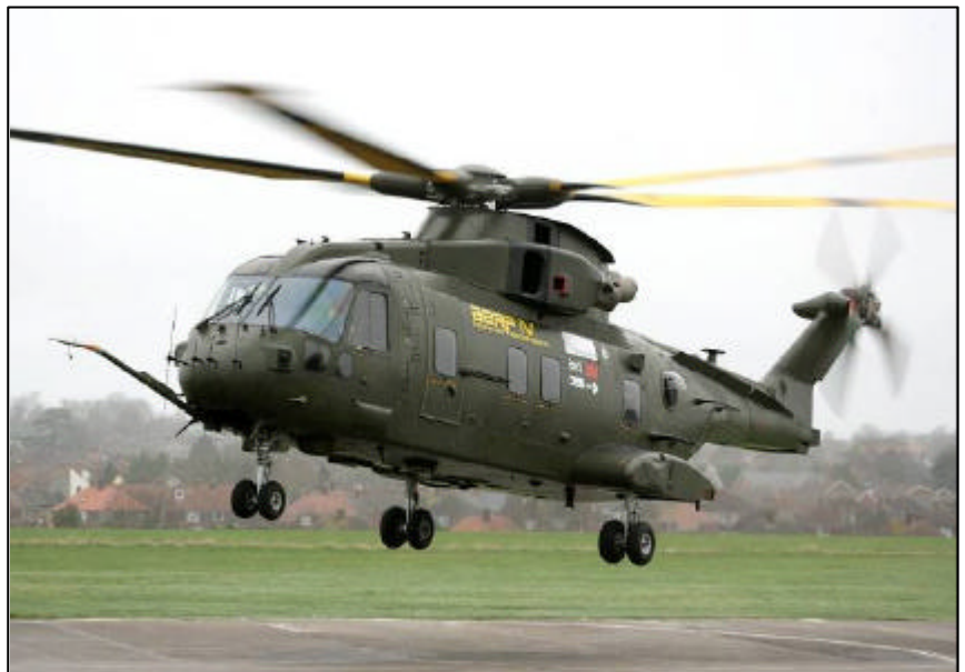
Figure 6. BERP IV Composite Main Rotor Blades on TDP trials aircraft RAF01. First Flight, 12 Jan 07, AgustaWestland, Yeovil
