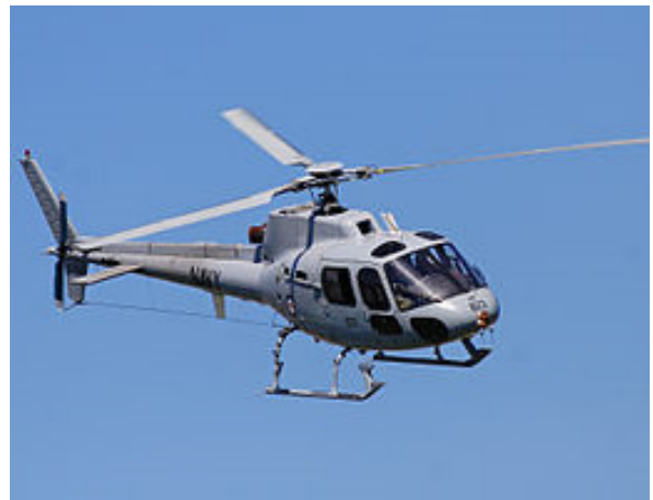
Figure 5: H125 : \sigma(0.054) , b(3) , DL( 25 \text{ kg/m}^2 ), U( 226,6 \text{ m/s} ), Neng( 1 ), Kpns( 1.15 ).
