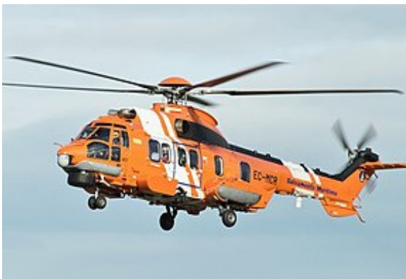
Figure 7: H225 : \sigma(0.108) , b(5) , DL(53 \text{ kg/m}^2) , U(224,78 \text{ m/s}) , Neng(2) , Kpns(1.25) .
