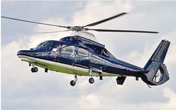
Figure 3: Dauphin AS365N : \sigma(0.086) , b(4) , DL( 35 \text{ kg/m}^2 ), U( 218,6 \text{ m/s} ), Neng( 2 ), Kpns( 1.2 ).
