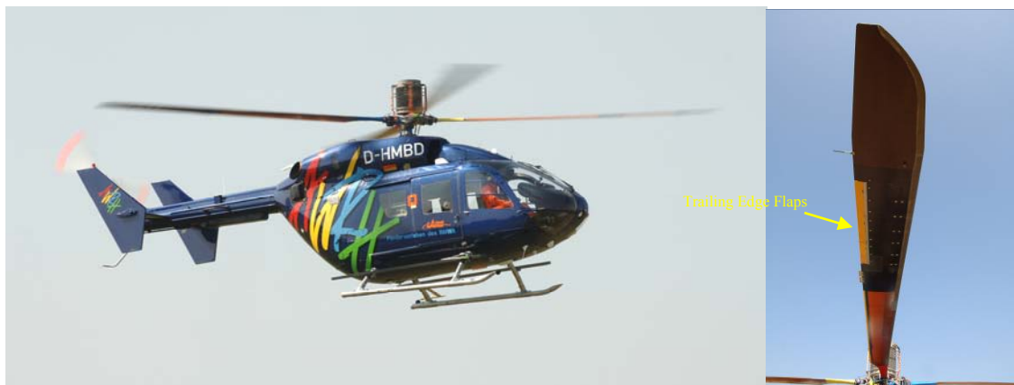
Figure 1. Experimental system featuring active rotor with trailing edge flaps
