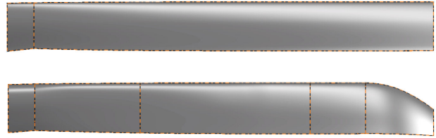
Figure 21: Comparison of the baseline XV15 blade geometry and the selected optimal P3.
