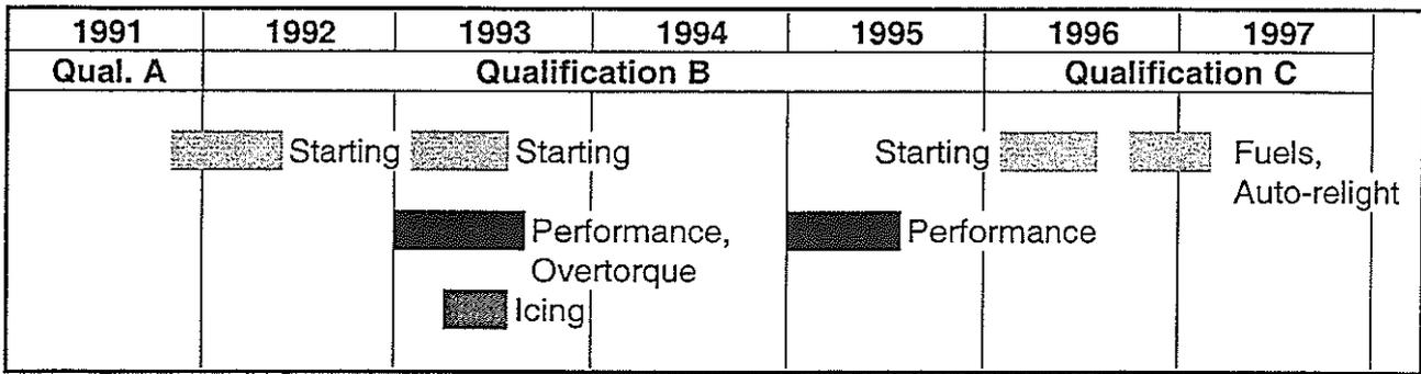
**Figure 3:** Time schedule for MTR390 qualification tests on the altitude test facility
