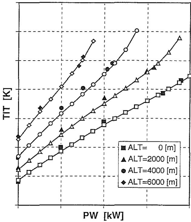
Figure 7: Model and test data at  $T_{s0} = -10$  °C from Qualification B
