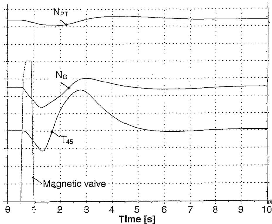
**Figure 6:** Demonstration of the auto-relight system function at ALT = -300 m and  $T_{s0} = -30\text{ }^{\circ}\text{C}$
