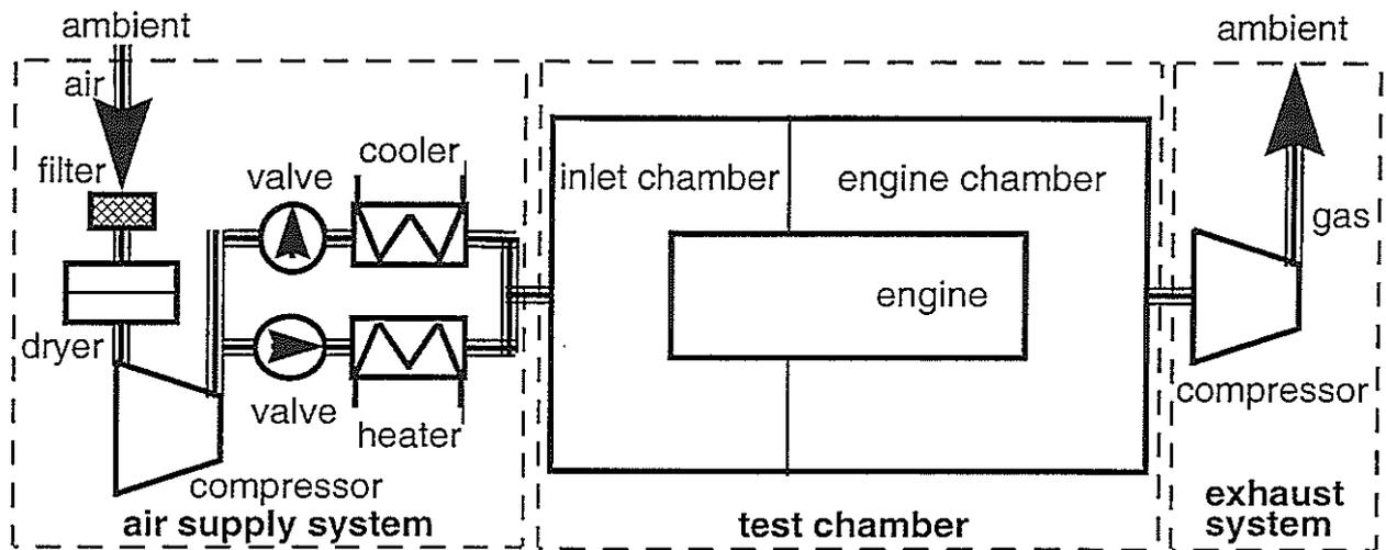
**Figure 2:** A schematic layout of an altitude test facility
