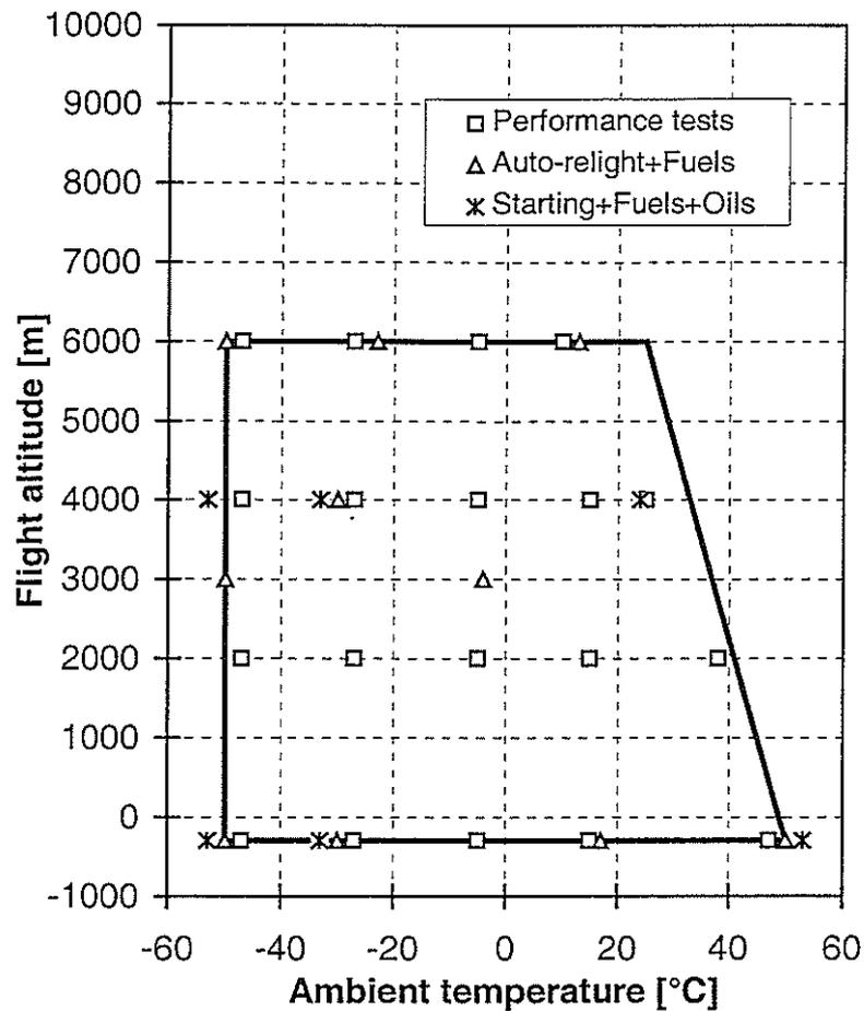
Figure 4: Test points in the flight envelope (Qualification C)
