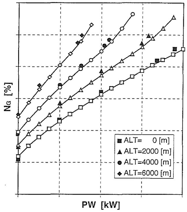
Figure 8: Model and test data at  $T_{s0} = -10$  °C from Qualification B
