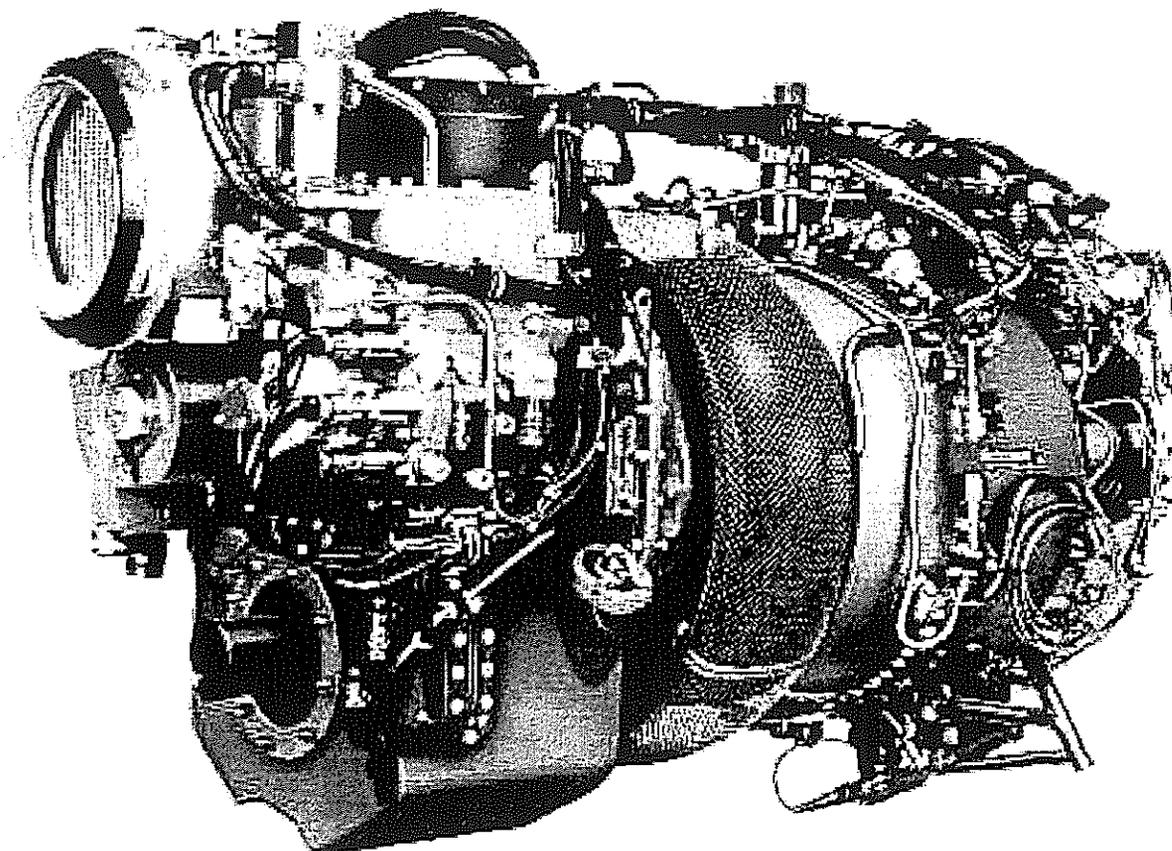
**Figure 1:** The MTR390 turboshaft engine
