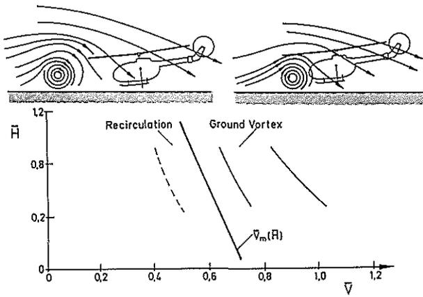
Figure 7: Boundary for Recirculation and Ground Vortex Regions
