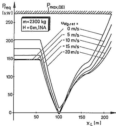
Figure 19: Power Required in Flare-Segment for Defined Flight Path
