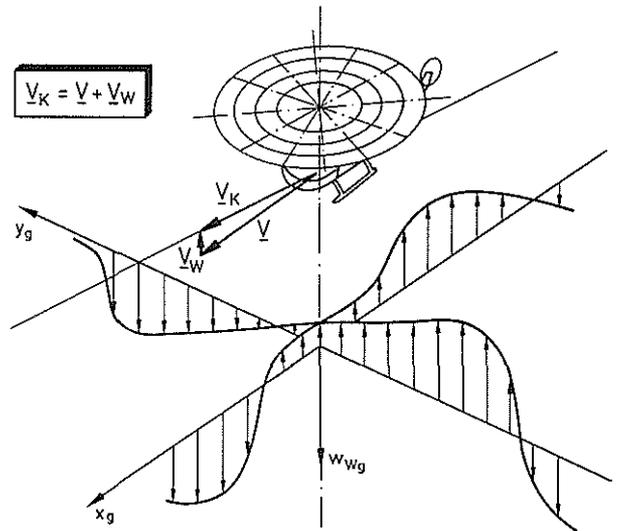
Figure 2: Penetration of a Vertical Wind Field with Varying Wind-Velocity
