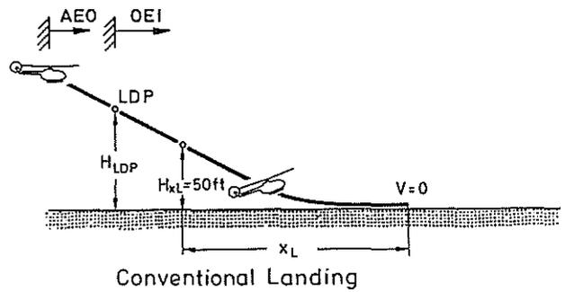
Figure 15: Takeoff- and Landing Profiles
