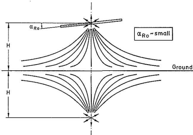
Figure 5: Source Model in Ground Effect
