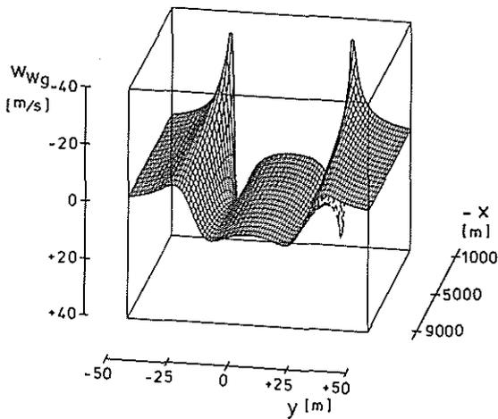
Figure 23: Induced Vertical Velocity Profile of B 747-Trailing-Vortices
