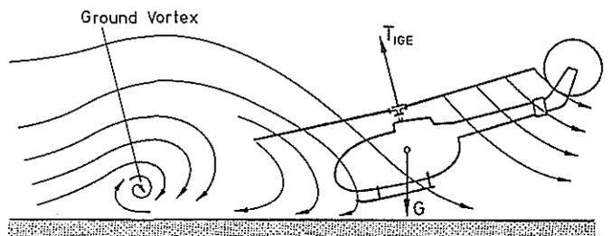
Figure 6: Helicopter in Ground Effect for Low Forward Speed
