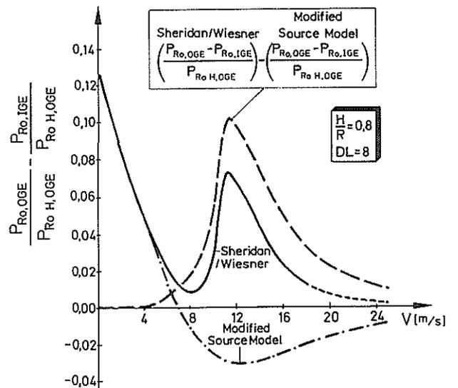
Figure 11: Non-Dimensional Main-Rotor-Power-Required-Difference between OGE- and IGE-Case
