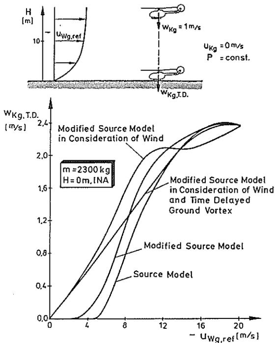
Figure 17: Influence of Ground Boundary Layer on Vertical Velocity at Touch Down for Descent ( $P = \text{const.}$ )
