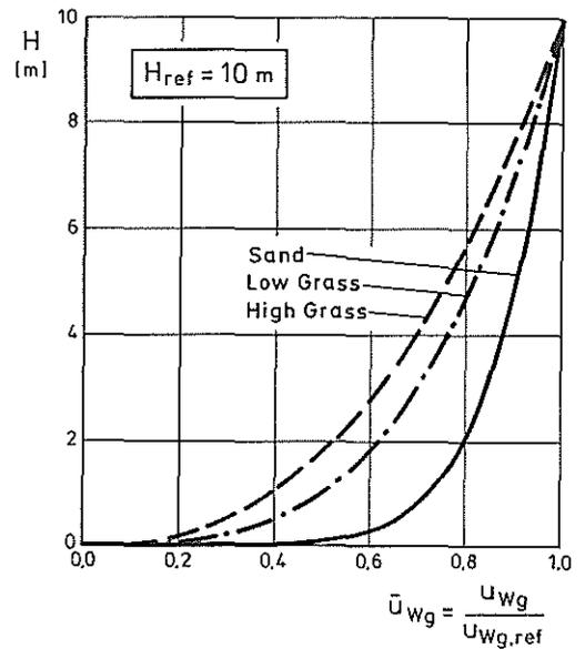
Figure 16: Non-Dimensional Horizontal Wind-Velocity as Function of Height and Surface-Roughness
