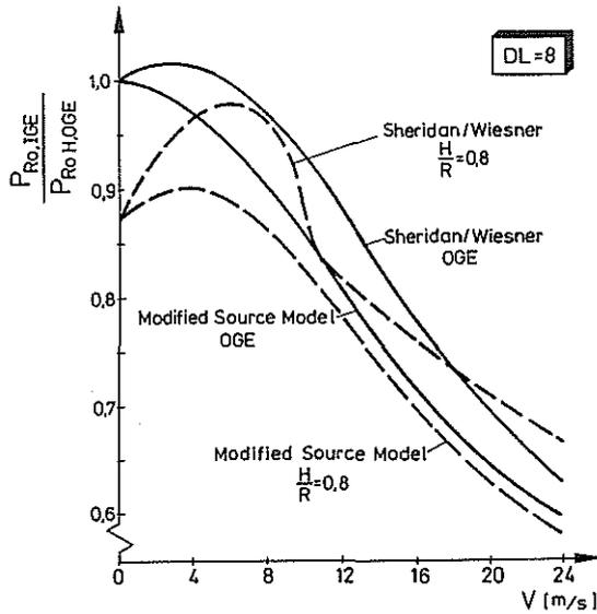
Figure 9: Non-Dimensional Main Rotor Power Required in Ground Effect
