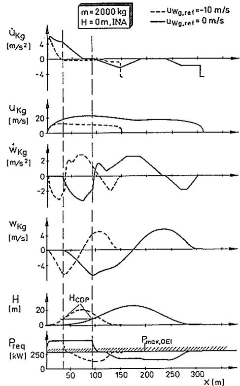
Figure 20: Wind Influence on Rejected Takeoff-Profile
