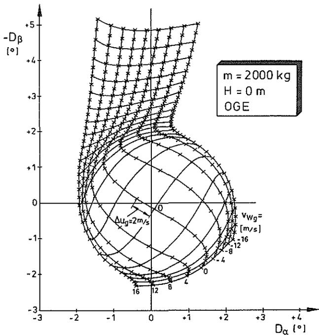
Figure 3: Cyclic Pitch Angle at Swashplate as Function of Airspeed
