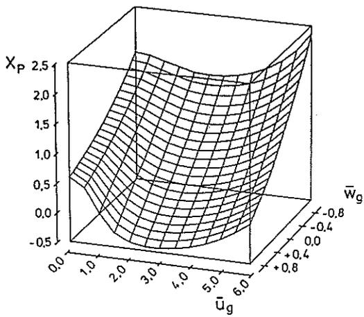
Figure 1: Power Factor at Forward Flight with Climb/Descent
