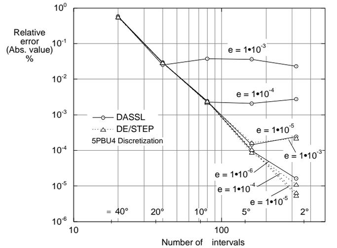
Figure 4: Absolute value of relative error as a function of  $\zeta$ -discretization, for both ODE solvers and several values of the local error tolerance  $e$ ; 5PBU4 discretization.
