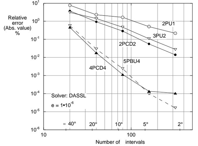
Figure 3: Absolute value of relative error as a function of  $\zeta$ -discretization; DASSL with  $e = 10^{-6}$ .
