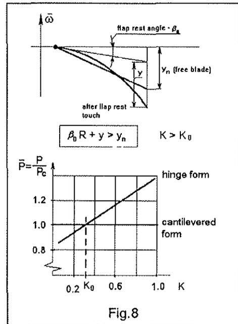
The clear understanding of the phenomenon provided the exact and reliable measures to be taken. A swash plate limit to back was reduced by 0.5° and a limiting condition for swash plate deflection was introduced particularly an additional force on control stick when a helicopter is on the ground warns a pilot to act with care. In flight the restriction is removed enabling the employment of full range longitudinal control and manoeuvring properties
