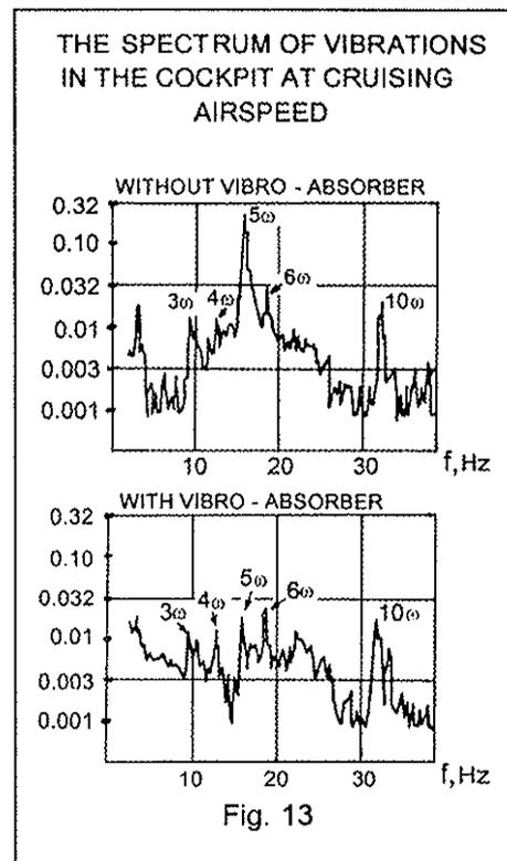
pilot involvement into the oscillation loop. It was proved the vibration has nothing to do with blades flutter. A supplementary instruction for crew to avoid, eliminate or prevent the vibration has been worked up.
