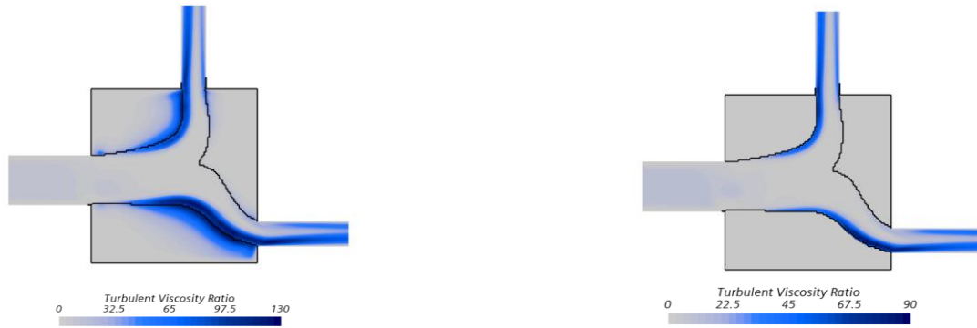
Figure 6: Comparison of the turbulence viscosity field between the basic model (left) and the improved one (right)
