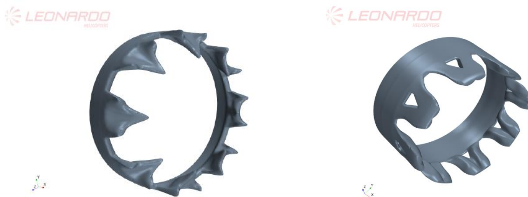
Figure 13: Reconstructed CAD geometries. Reconstruction process did not take into account for small asymmetries
