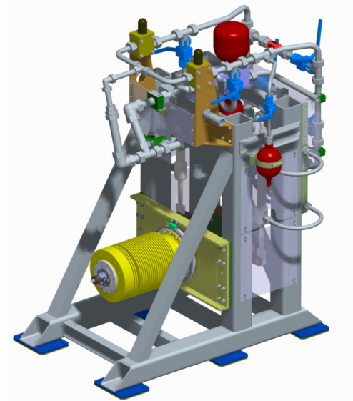
Figure 28: EMA test rig for functional and load testing
