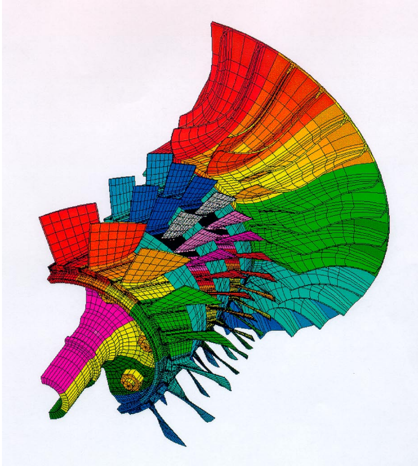
Figure 7- 3-D Finite Element (FE) Model of PT6T-3D Compressor
