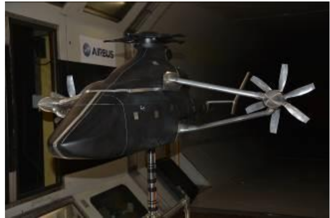
Fig. 25: Performance and Handling Qualities mock-up at Airbus Filton Wind Tunnel – configuration with active propellers
