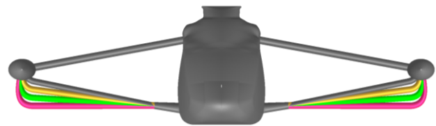
Fig. 21: Explored settings of tip wing gap and lower wing dihedral.
