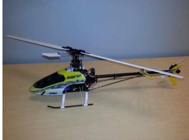
Figure 11: RC helicopter used for load/strain data acquisition testing
