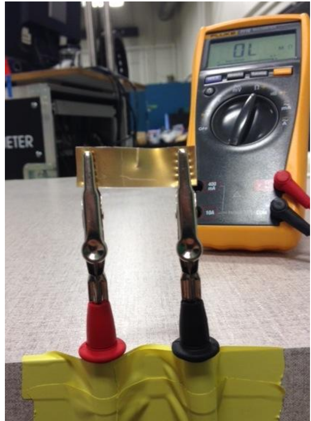
Figure 7: Damaged Metal Rubber rectangular test specimen experimental test setup
