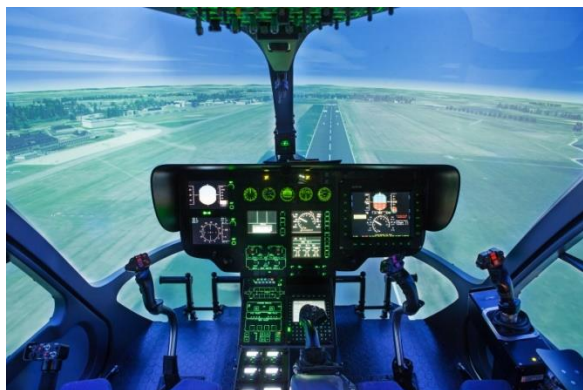
Figure 5: Simulation Cockpit of Active Control Technology/Flying Helicopter Simulator (ACT/FHS)
