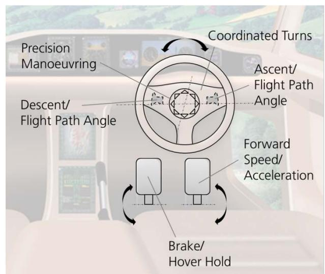
Figure 3. Steering wheel in combination with rocker switches for height control.
