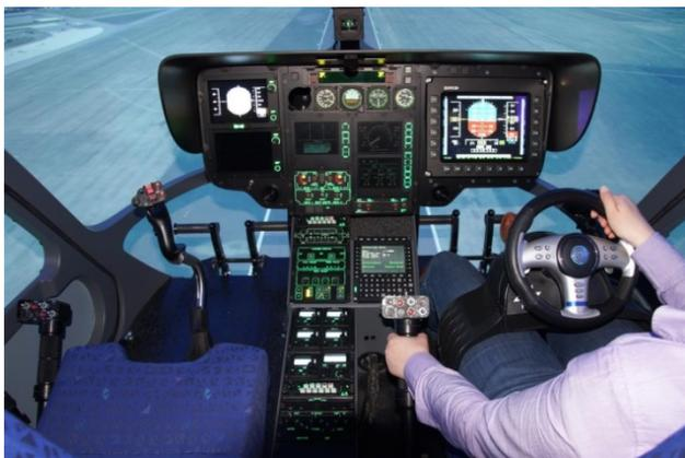
Figure 5. AVES EC135 cockpit featuring conventional and steering wheel inceptors.
