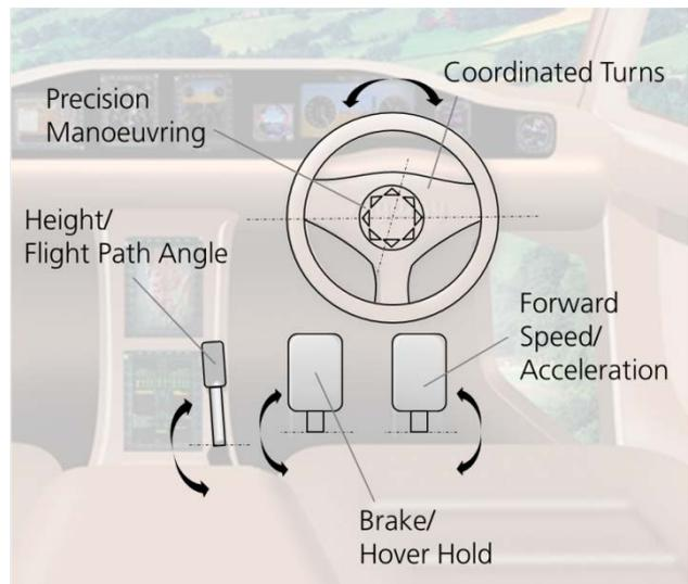
Figure 2. Steering wheel control concept including collective lever.
