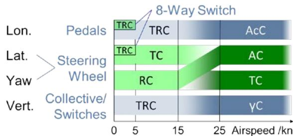
Figure 4. Speed dependent control laws for steering wheel usage.
