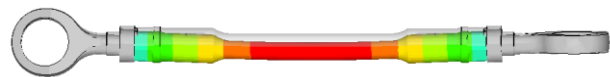
Figure 17: Residual deformation of the serial main pitch rod obtained with RADIOSS superimposed with the initial shape (shadow)
