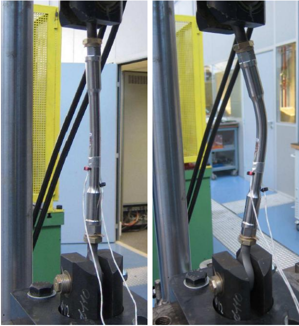
Figure 20: Main rotor pitch rod on the buckling bench test (at the beginning and at the end of the test)
