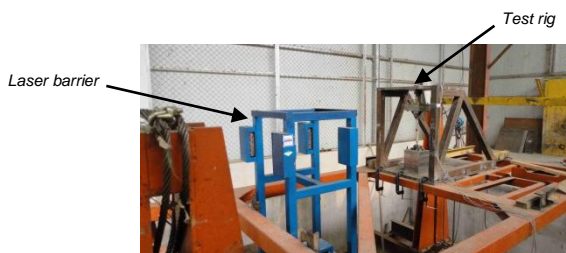
Figure 4: Laser barrier and test bench
