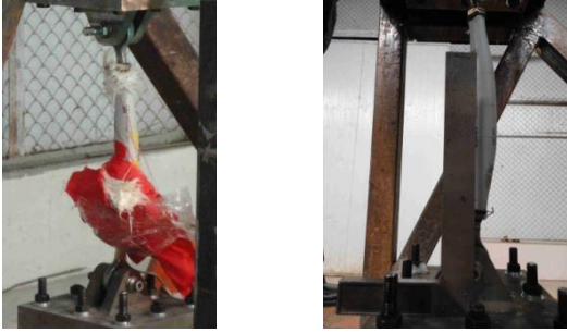
Figure 8: Permanent deformation of the tested pitch rod
