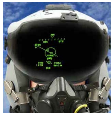
Figure 1: Vision Systems International Joint Helmet-Mounted Cueing System (JHMCS) for Fixed-Wing Fighter Aircraft
