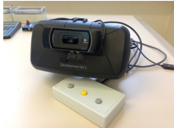
Figure 4: Low cost display demonstrator Oculus DK 2 coupled with a Logitech camera (B910) for simulating “looking -through” capability.
