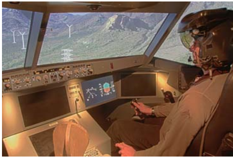
Figure 6: JedEye HMD integrated into Generic Cockpit Simulator GECO together with cyclic and collective sticks for helicopter flight simulation.
