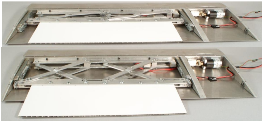
Figure 2: Chord increase through the use of extendable Trailing-Edge Plate (TEP) shown in retracted (above), and extended (below) configurations (top skin removed in figure)
