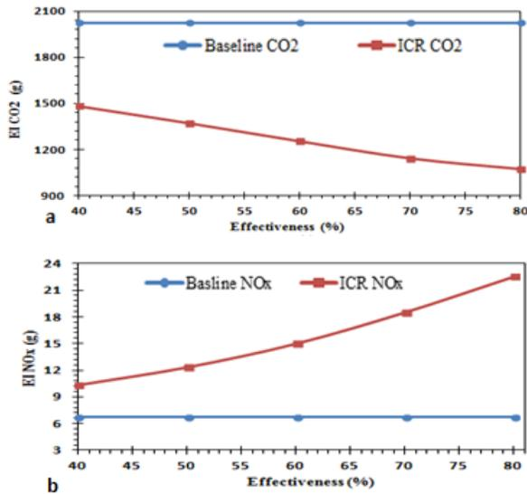
Figure 15: (a) Emitted CO<sub>2</sub>, (b) Emitted NO<sub>x</sub> for TEM, Baseline Simple Cycle and ICR rotorcraft, SAR Mission
