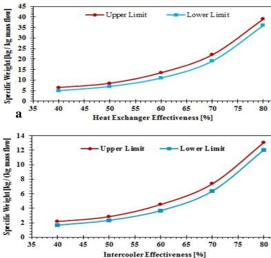
Figure 4: (a) Fixed geometry tubular type heat exchanger specific weight correlation adopted from<sup>(14)</sup>, (b) Intercooler specific weight correlation.
