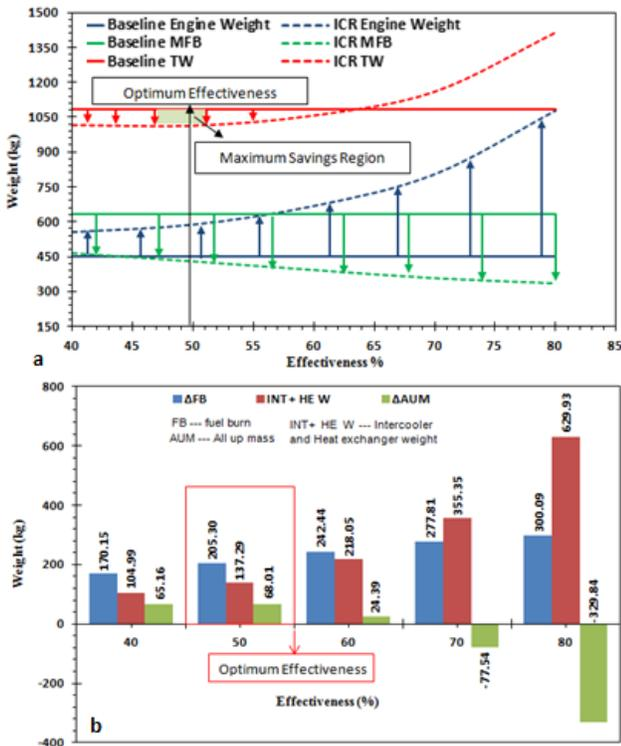
Figure 16: (a) ICR tradeoff study, Oil and gas mission; (b) ΔAUM for conceptual ICR rotorcraft.
