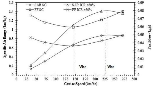
Figure 7: Specific Air Range for Baseline Engine A1 and ICR Engine B1 helicopter with 60% HE effectiveness.
