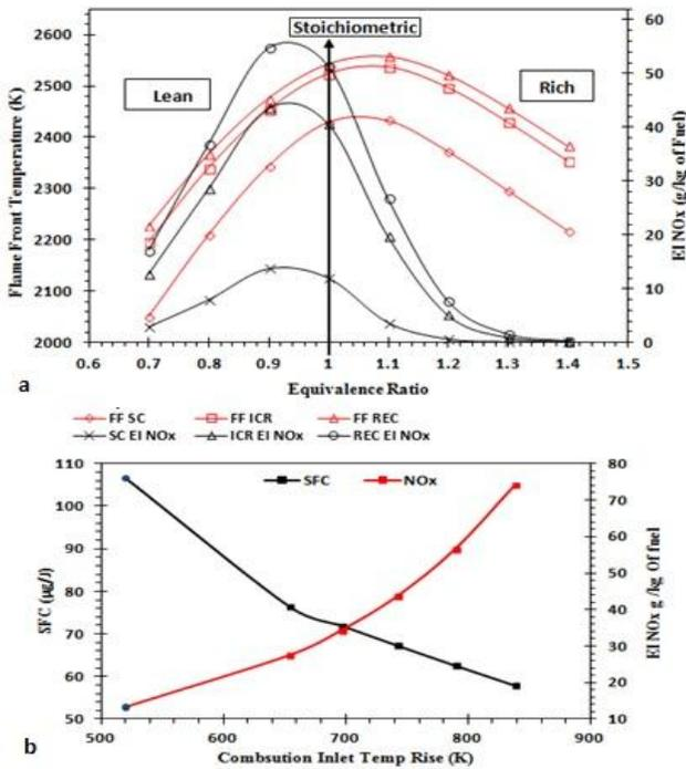
Figure 8: (a) EI  $\text{NO}_x$  and combustor equilibrium temperature Vs Equivalence Ratio, Engine A1 and ICR Engine B1; (b) SFC & EI  $\text{NO}_x$  vs inlet temperature Engine A1 and ICR Engine B1, at design point, points denoted by circles imply Engine A1.
