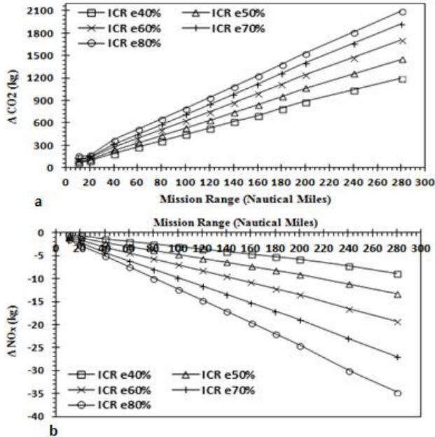
Figure 12: (a) Delta CO<sub>2</sub> Vs Mission Range for TEM ICR helicopter; (b) Delta NO<sub>x</sub> Vs Mission Range for TEM ICR helicopter.
