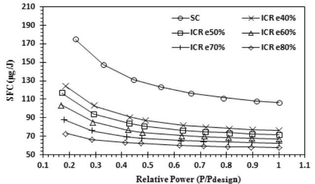
Figure 5: SFC vs ( $P/P_{\text{Design}}$ ) for Baseline Engine A1 and ICR Engine B1.
