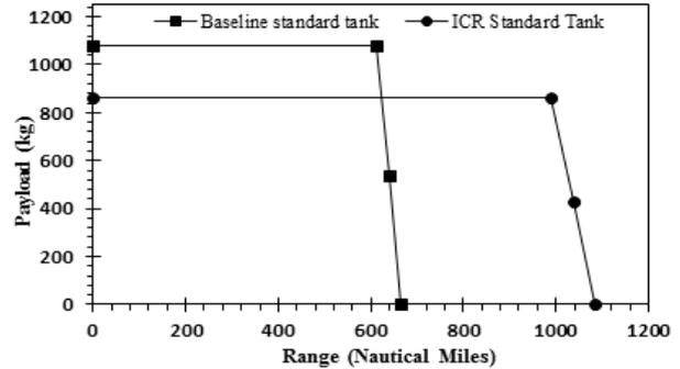
Figure 13: Payload-range diagram for Reference SA330 and regenerated helicopter
