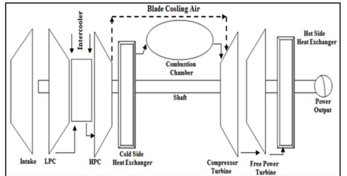
Figure 2: Schematic layout of a single-spool Intercooled Recuperated Turboshaft.
