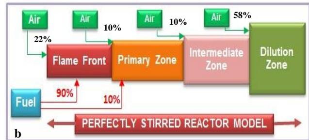
Figure 3: (a) Generic TURMO IV-C Combustor Model isometric view; (b) Combustor Zones and Reactor Models assumed for  $\text{NO}_x$  modeling of rotorcraft.
