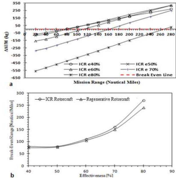
Figure 11: (a). Delta All-Up-Mass Vs Mission Range for TEL regenerated helicopter. (b). Break-even Range for TEM ICR and Recuperated helicopter
