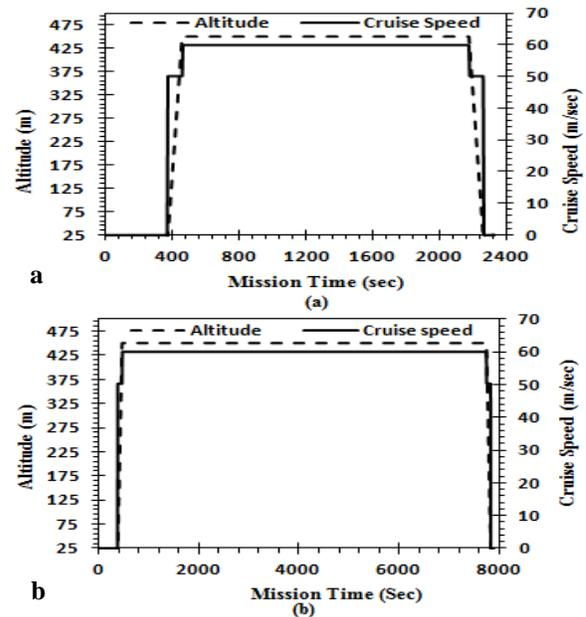
Figure 9: (a) Time variations of deployed operational airspeed and AGL altitude for mission range of 60 nautical mile; (b) Time variations of deployed operational airspeed and AGL altitude for mission range of 240 nautical miles.
