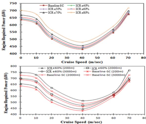
Figure 6: Reference SA330 PUMA and conceptual ICR helicopter, power vs cruise speed sea level and various altitudes
