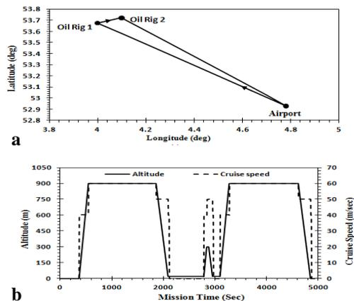
Figure 14: Oil and Gas mission: (a) geographical global coordinates; (b) time variations of operational airspeed and AGL altitude.
