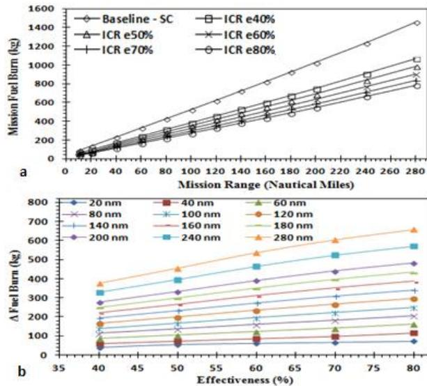
Figure 10: (a). Mission fuel burn Vs mission range for simple cycle and ICR helicopter; (b) Delta Fuel burn Vs HE Effectiveness for TEM ICR for simulated missions.
