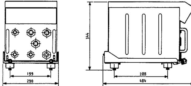
**Fig. 9 - PROCESSOR LAYOUT**
