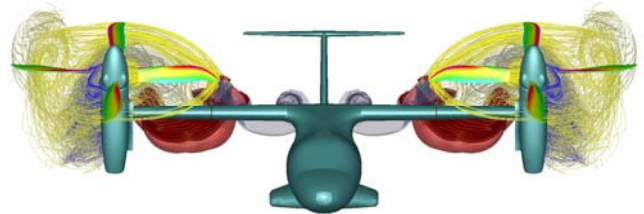
Figure 5. ADPANEL CVC wake development of the ERICA Innovative Tiltrotor in descent flight condition
