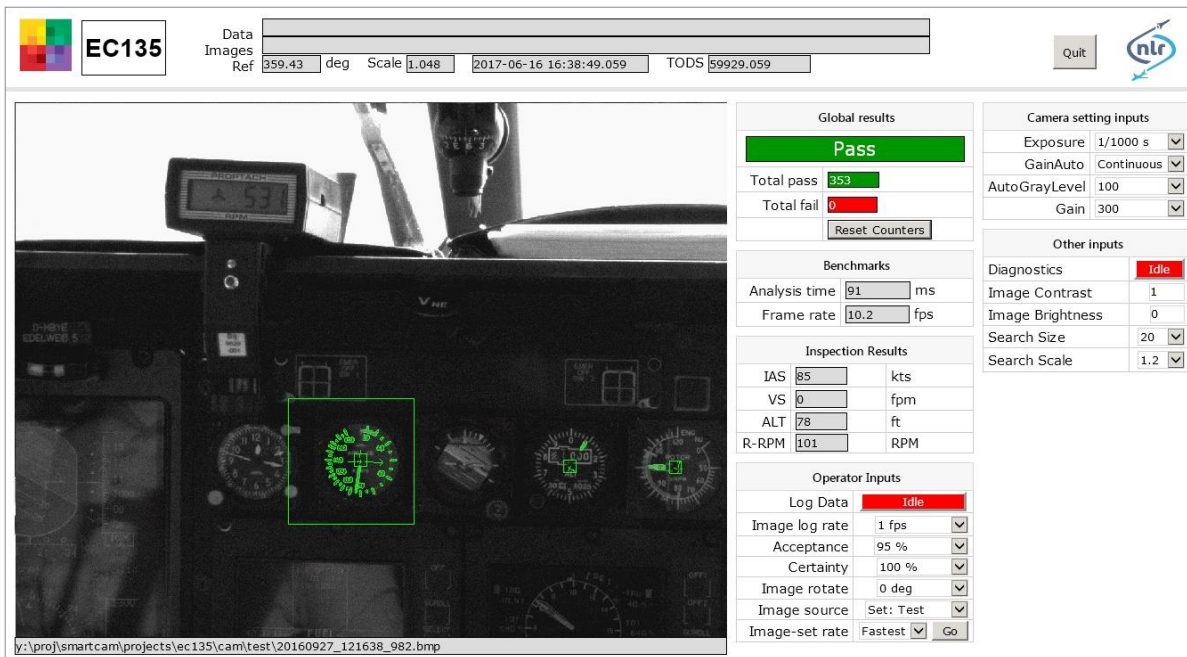
Figure 4: Smartcam operator interface showing the digitisation of the airspeed, altitude and vertical speed indicators.
