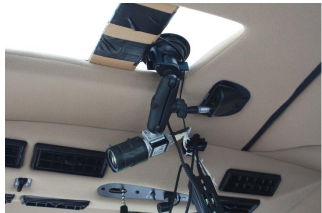
Figure 3: Smartcam as installed on R66.
