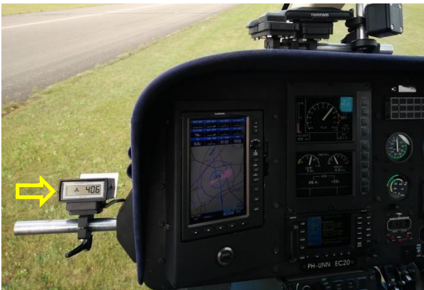
Figure 2: Optical tachometer as installed on EC120.
