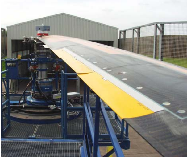
Fig. 23 Flap rotor blade on the Whirl tower
