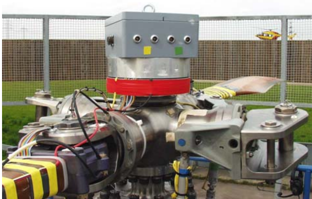
Fig. 24 BK117 hingeless rotor hub with signal processing electronics on the whirl tower
