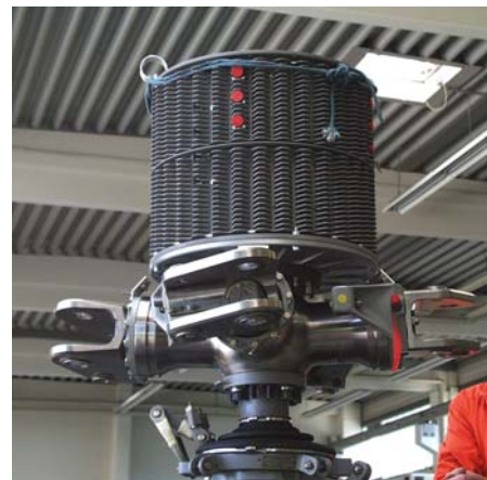
Fig. 36 Hub electronic compartment during a test installation on the helicopter
