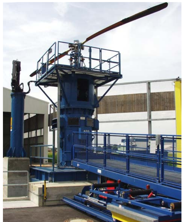
Fig. 22 ECD test stand for main rotors
