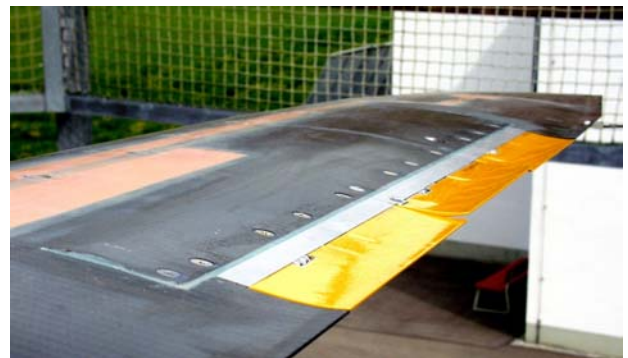
Fig. 1 EC145 full scale rotor blade with piezoelectric actuated trailing edge flaps
