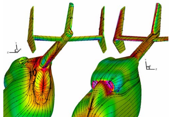
Figure 20: Surface pressure distribution and surface friction lines on fuselage of EC 145 helicopter (ref. [12], with permission)
