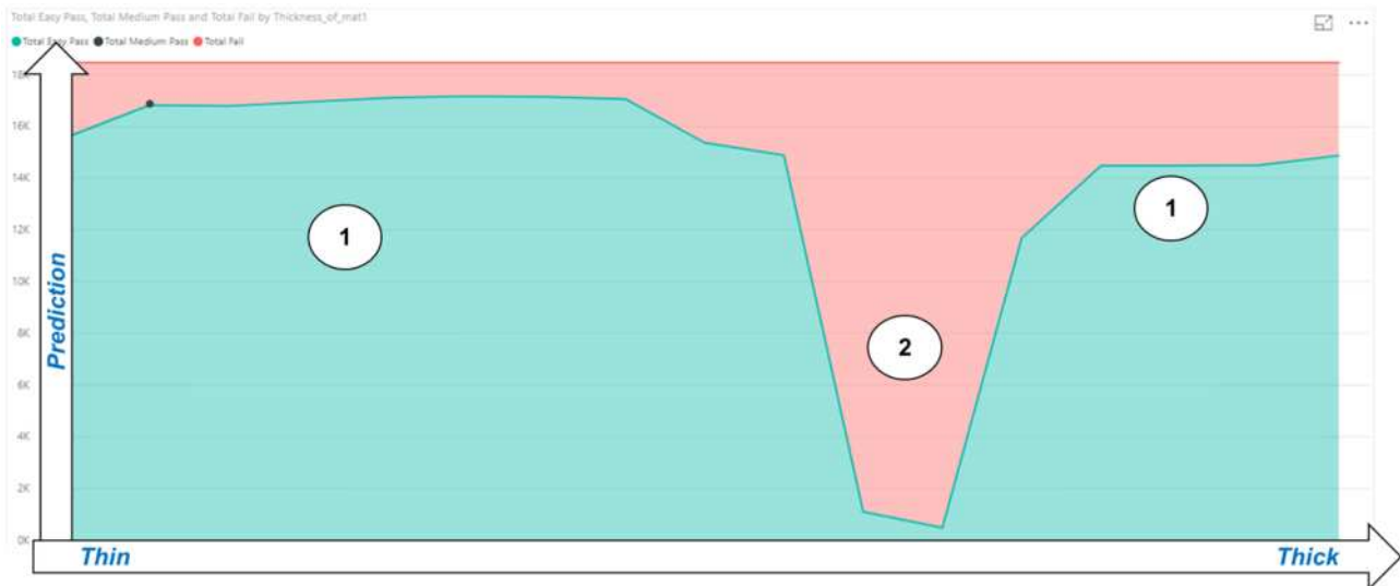
Fig 6. Prediction of Fail (red), Easily Pass (green) depending the thickness of reinforced epoxy laminates for 60s vertical tests, afterflame time criteria.
