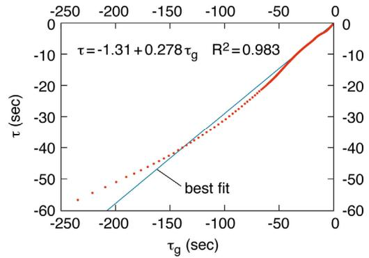
**Fig 3 Regression fit of  $\tau$  vs  $\tau_g$  for helicopter in acceleration-deceleration manoeuvre (Ref 10)**
