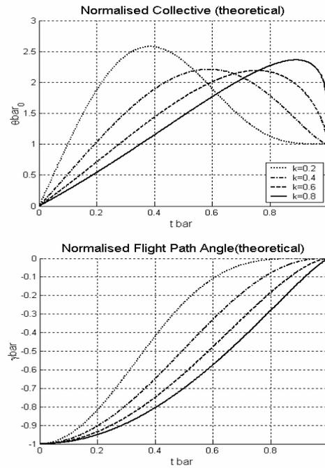
**Fig 15 Normalised collective pitch and flight path response following a constant acceleration  $\tau$  guide**
