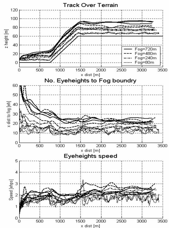
**Fig 7 Flight trajectories and eye-height parameters for terrain hugging manoeuvres**
