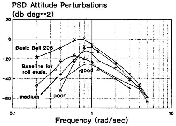
Figure 7: Pitch Axis Attitude Perturbation PSDs ( $\delta\theta$ )
