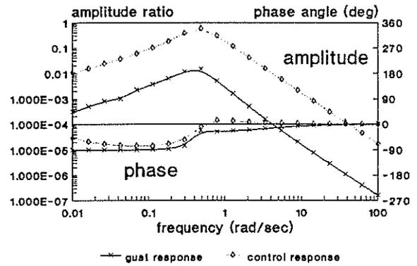
Figure 4: Pitch Axis Control and Gust Response Transfer Functions
