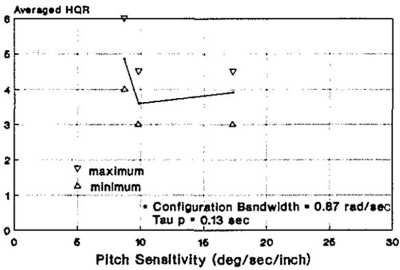
Figure 18: Effect of Sensitivity on Low Bandwidth Pitch Model Handling Qualities
