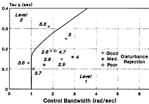
Figure 10: Pitch Axis Results Quickstop Task
