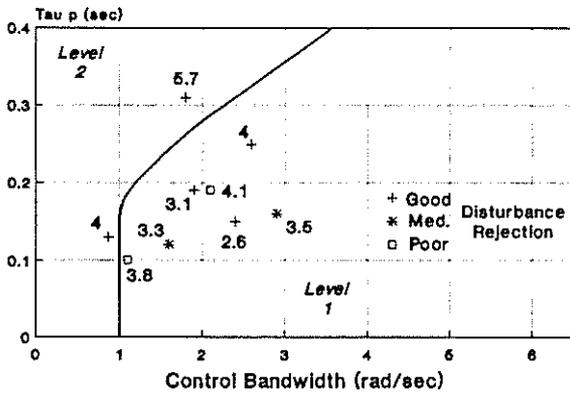
Figure 8: Pitch Axis Results Hover & Landing Tasks
