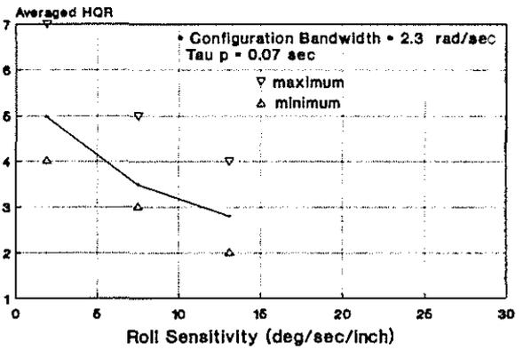
Figure 19: Effect on Sensitivity on High Bandwidth Pitch Model Handling Qualities
