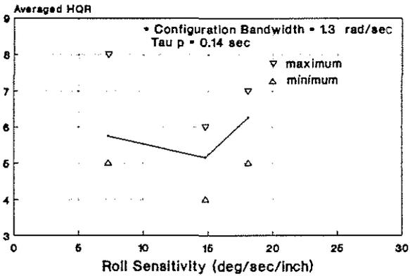
Figure 20: Effect on Sensitivity on Low Bandwidth Roll Model Handling
