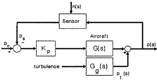
Figure 1: Simple Rate Feedback Architecture
