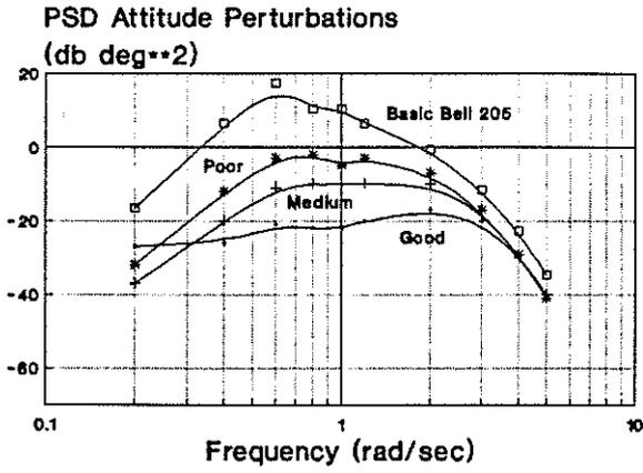
Figure 6: Roll Axis Attitude Perturbation PSDs ( $\delta\phi$ )
