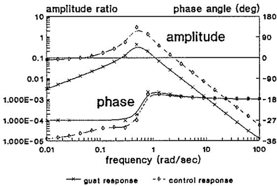
Figure 3: Roll Axis Control and Gust Response Transfer Functions
