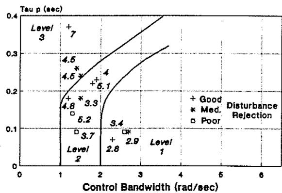
Figure 11: Roll Axis Results Hover & Landing Tasks
