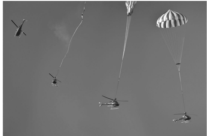
Figure 15: Parachute ejection phases (courtesy of Curti Aerospace Division).
