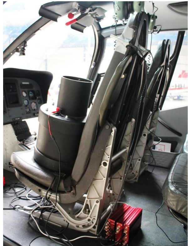
Figure 2 – Measurement setup during transfer path scanning measurements
